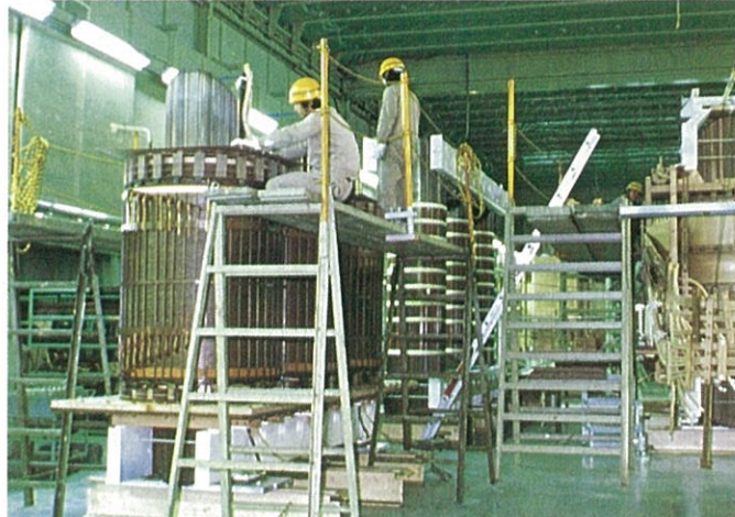
▼ (b) Assembling of active parts in dust-proof air-conditioned room
