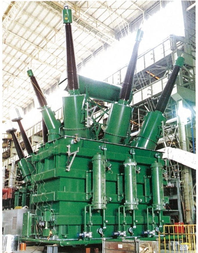
Photo 12 Forced-oil water-cooled outdoor transformer of three-phase 60Hz 500MVA and 24/432kV
