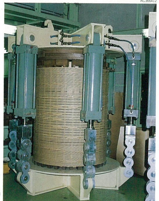
Photo 13 Pretightening of coil
