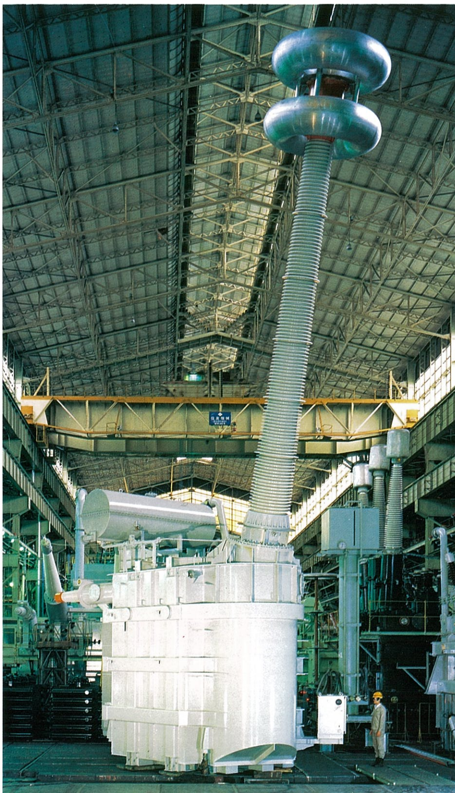
Photo 1 UHV Testing-transformer single phase \frac{1550}{\sqrt{3}} kV 50Hz
