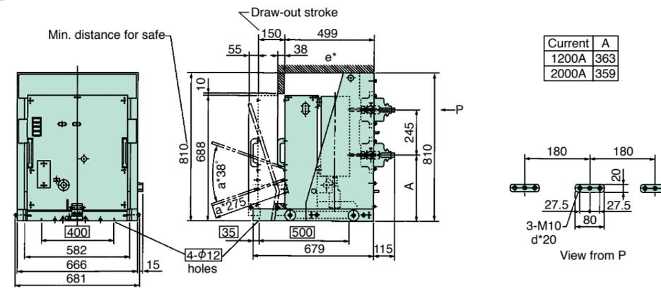
Note\* a: approx. d: depth e: elec. parts equal to earth potential h: height p: pitch
