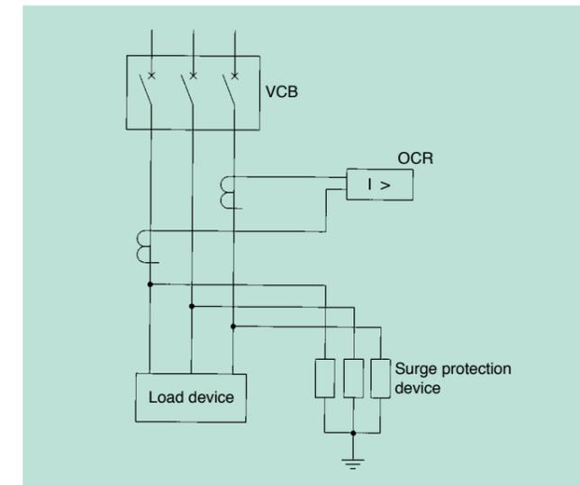
When using a C-R suppressor, it may be necessary to use a directional relay as a ground fault protection relay. Note that the C-R suppressor may be damaged due to higher harmonics.
