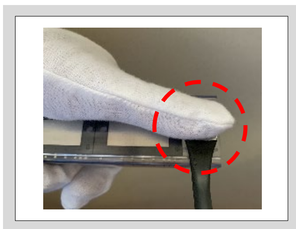
Fig. 2-5 How to hold the pin
