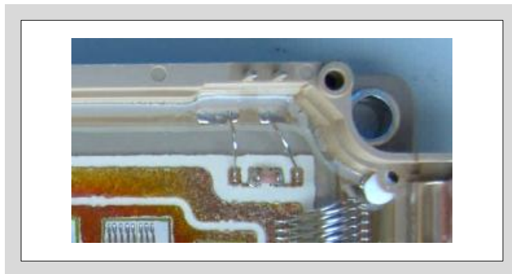
Fig.1 Example of the internal structure of an IGBT module with a NTC thermistor
