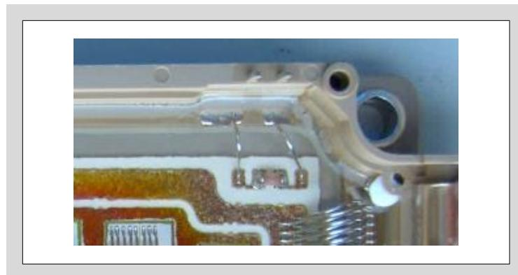
Fig.1 Example of the internal structure of an IGBT module with a NTC thermistor
