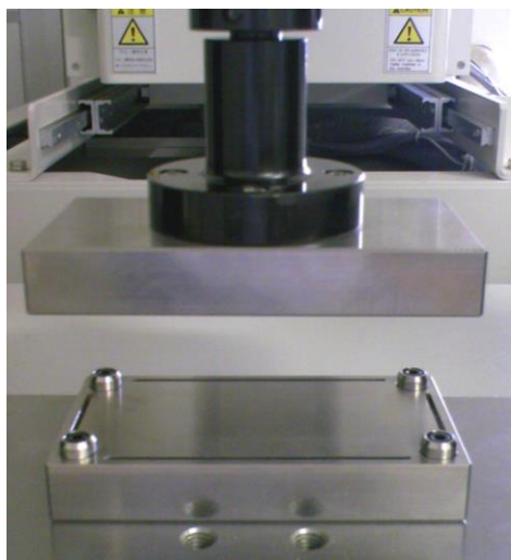
(a) Set the press-in upper tool and lower tool on the press machine.
