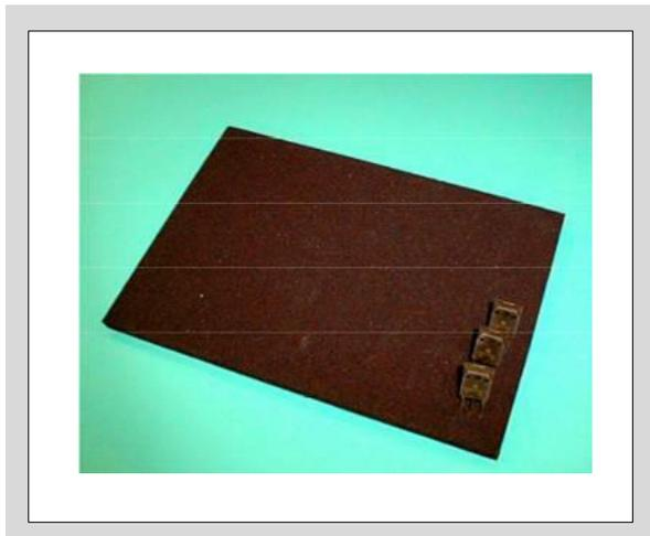
Figure 6-5. Conductive foam
