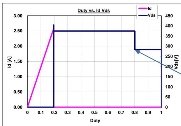
If the Vds waveform has a step, the mode becomes Discontinuous.
