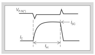
Fig.1 Definition of  $I_{SC}$  and  $t_{SC}$
