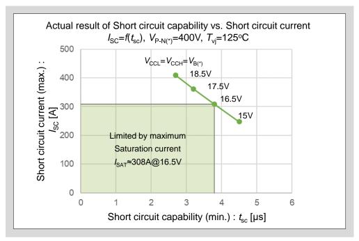
Fig.5 6MBP35XSD(F)060-50 Short circuit capability and SCSOA
