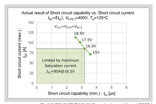
Fig.2 6MBP15XSD(F)060-50 Short circuit capability and SCSOA
