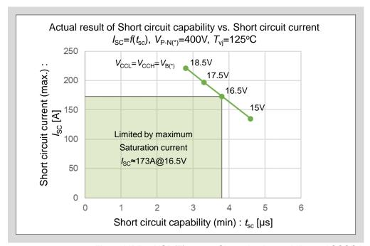
Fig.4 6MBP30XSD(F)060-50 Short circuit capability and SCSOA
