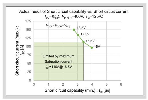
Fig.3 6MBP20XSD(F)060-50 Short circuit capability and SCSOA
