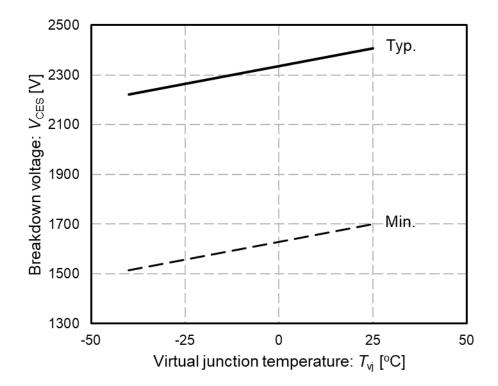
In general, semiconductor devices, the lattice vibration in silicon crystals decreases as temperature decreases and the collision of carriers is suppressed. And the impact ionization ratio is increased and the breakdown voltage of semiconductor devices becomes lower. Therefore when you use the module at low temperature, please take into account the reduction of the breakdown voltage in your design.
