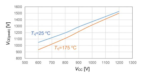
Conditions:  $R_G$ =1.2  $\Omega$ ,  $I_C$ =800 A,  $V_{GE}$ =15 V/-15 V,  $L_S$ =35 nH
