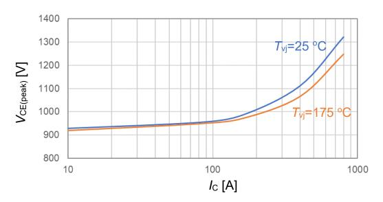
Conditions:  $R_G$ =1.2  $\Omega$ ,  $V_{CC}$ =900 V,  $V_{GE}$ =15 V/-15 V,  $L_S$ =35 nH
