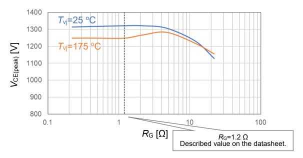
Conditions:  $I_C$ =800 A,  $V_{CC}$ =900 V,  $V_{GE}$ =15 V/-15 V,  $L_S$ =35 nH
