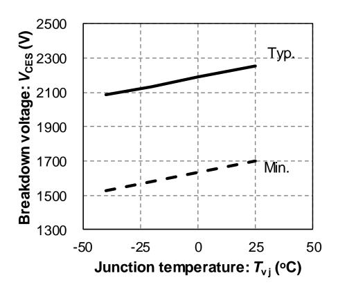
In general, semiconductor devices, the lattice vibration in silicon crystals decreases as temperature decreases and the collision of carriers is suppressed. And the impact ionization ratio is increased and the breakdown voltage of semiconductor devices becomes lower. Therefore when you use the module at low temperature, please take into account the reduction of the breakdown voltage in your design.
