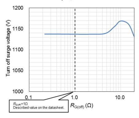
Measured condition:  $V_{cc}$ =900V,  $V_{GE}$ =15V/-15V,  $L_s$ =35nH,  $T_{vj}$ =25°C,  $I_F$ =12A, 600A,  $R_G$ =var.
