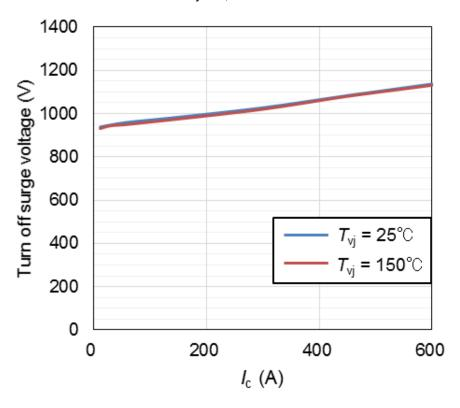
Measured condition:  $V_{cc}$ =900V,  $V_{GE}$ =15V/-15V,  $R_{G}$ =1 $\Omega$ ,  $L_{s}$ =35nH,  $T_{vj}$ =25°C, 150°C,  $I_{F}$ =var.
