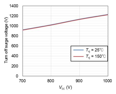
Measured condition:  $I_F$ =600A,  $V_{GE}$ =15V/-15V,  $R_G$ =1 $\Omega$ ,  $L_s$ =35nH,  $T_{vj}$ =25°C, 150°C,  $V_{cc}$ =var.
