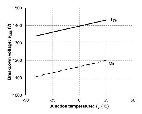
In general, semiconductor devices, the lattice vibration in silicon crystals decreases as temperature decreases and the collision of carriers is suppressed. And the impact ionization ratio is increased and the breakdown voltage of semiconductor devices becomes lower. Therefore when you use the module at low temperature, please take into account the reduction of the breakdown voltage in your design.
