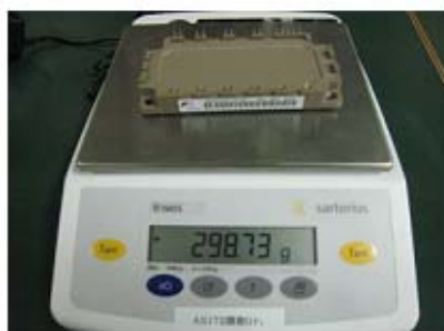
2. Measure weight of IGBT
