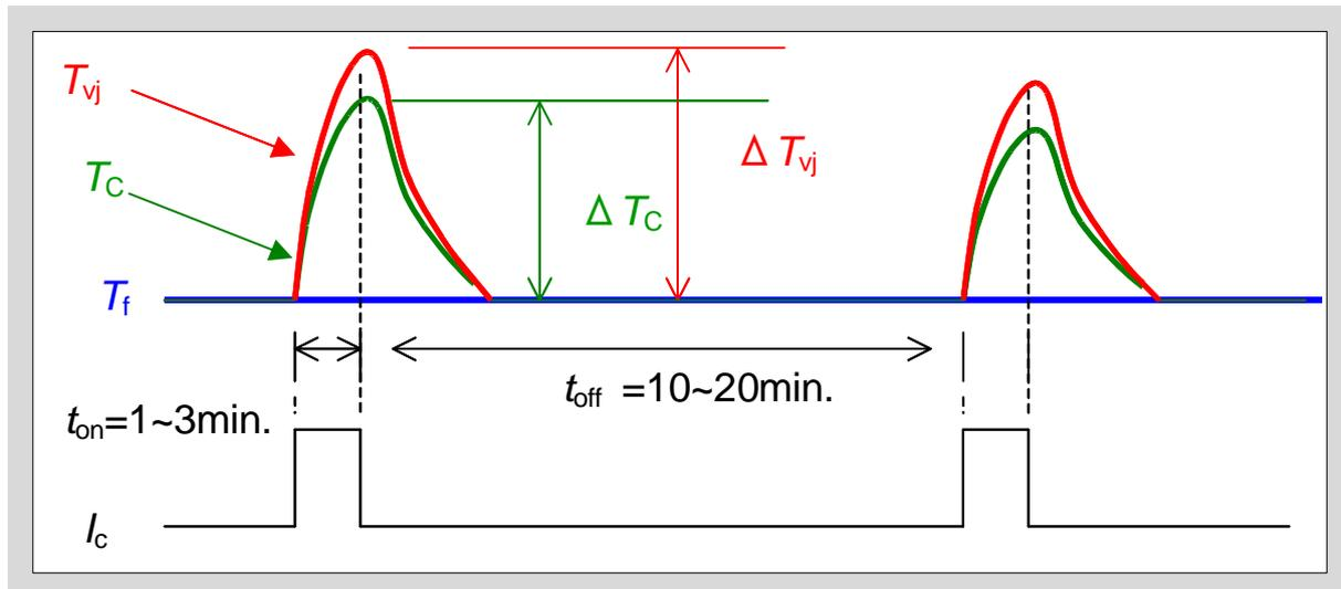
Fig. 11-7  $\Delta T_C$ -P/C test current pattern and temperature changes
