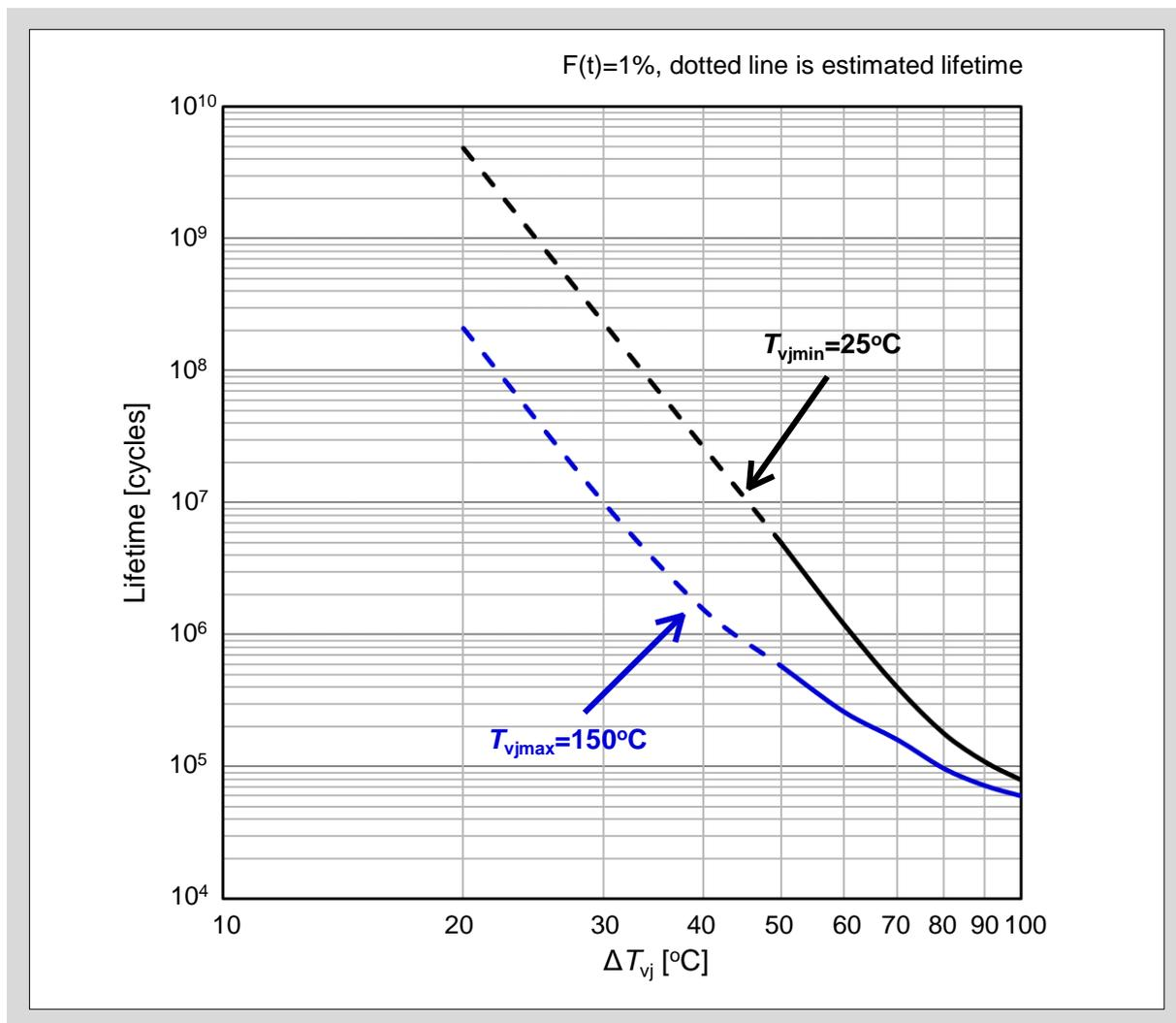
Fig. 11-5 Example of  $\Delta T_{vj}$ -P/C lifetime curve
