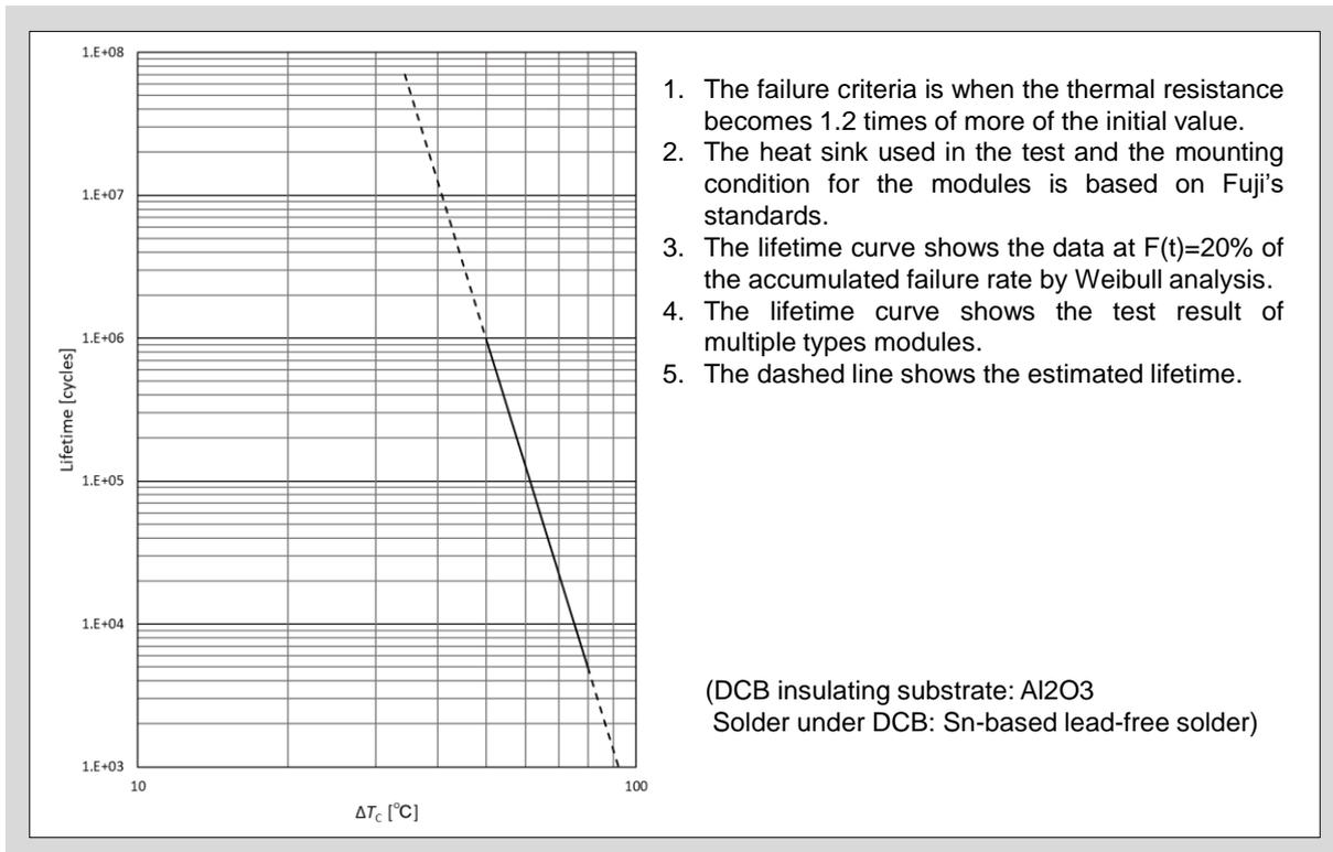
Fig. 11-9 Example of  $\Delta T_c$ -PC lifetime
