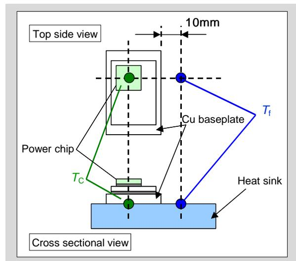
Fig. 11-4  $T_C$  and  $T_f$  measurement positions
