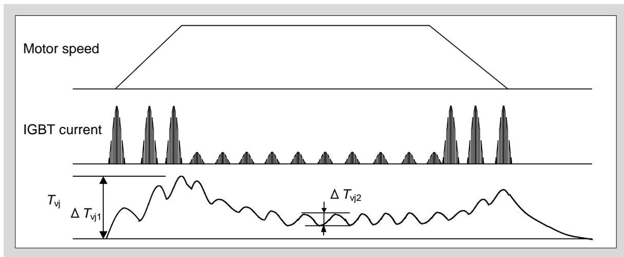
Fig. 11-6 Operation in actual equipment (example)
