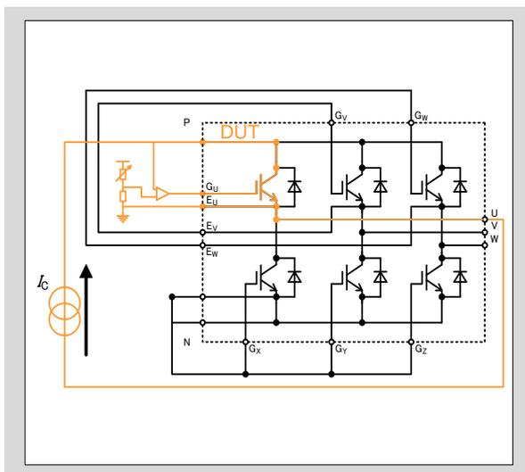
Fig. 11-3 Equivalent test circuit for  $\Delta T_{vj}$ -PC test
