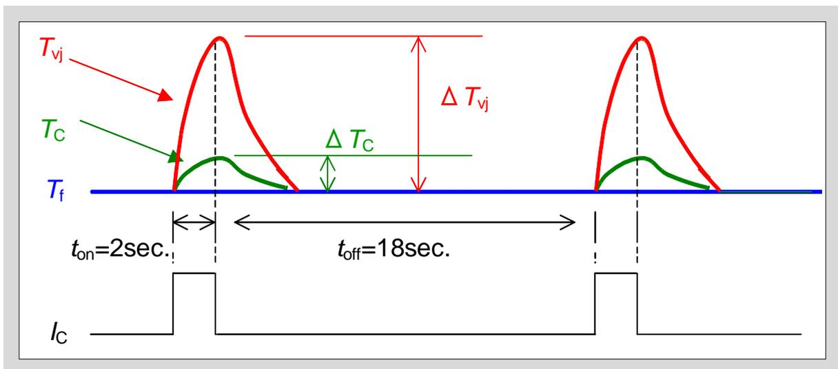
Fig. 11-2  $\Delta T_{vj}$ -P/C test current pattern and temperature changes
