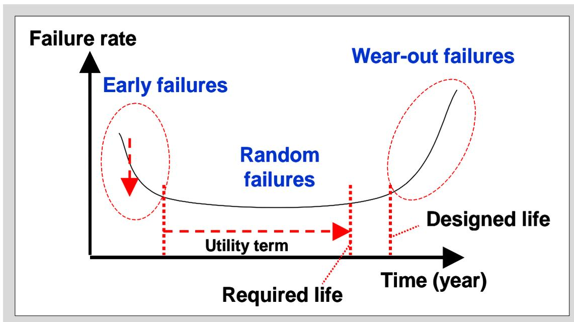
Fig. 11-1 Change in failure rate of semiconductor devices over time
