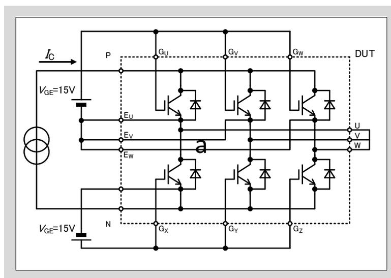
Fig. 11-8 Equivalent test circuit for  $\Delta T_C$ -P/C test
