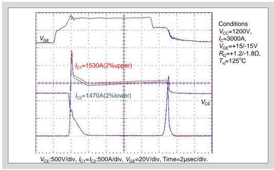
Fig. 8-10 Switching waveforms of two 1700V/1000A 2-Pack modules connected in parallel
