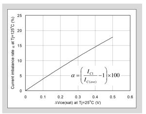
Fig. 8-1 Example of different output characteristics
