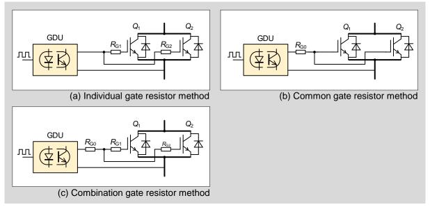
Fig. 8-13 Gate resistor configuration in common driver method
