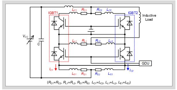
Fig. 8-9 Equivalent circuit when paralleling two 2-Pack modules
