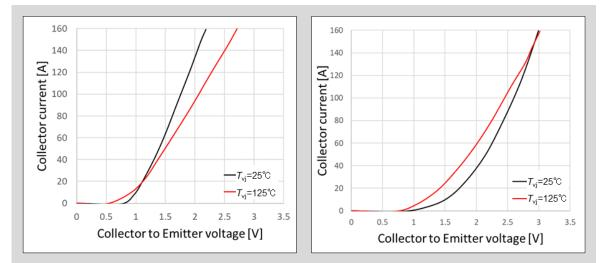
Fig. 8-5 Comparison of IGBT output characteristics (left: positive  $T_{vj}$  dependency, right: negative  $T_{vj}$  dependency)
