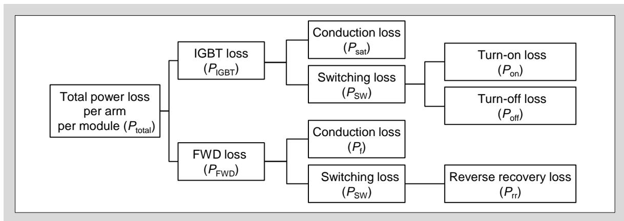
Fig. 6-2 Classification of IGBT module power loss
