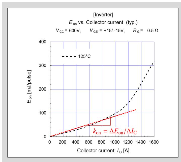
Fig. 6-6 Approximation of  $I_C$  dependence of switching energy
