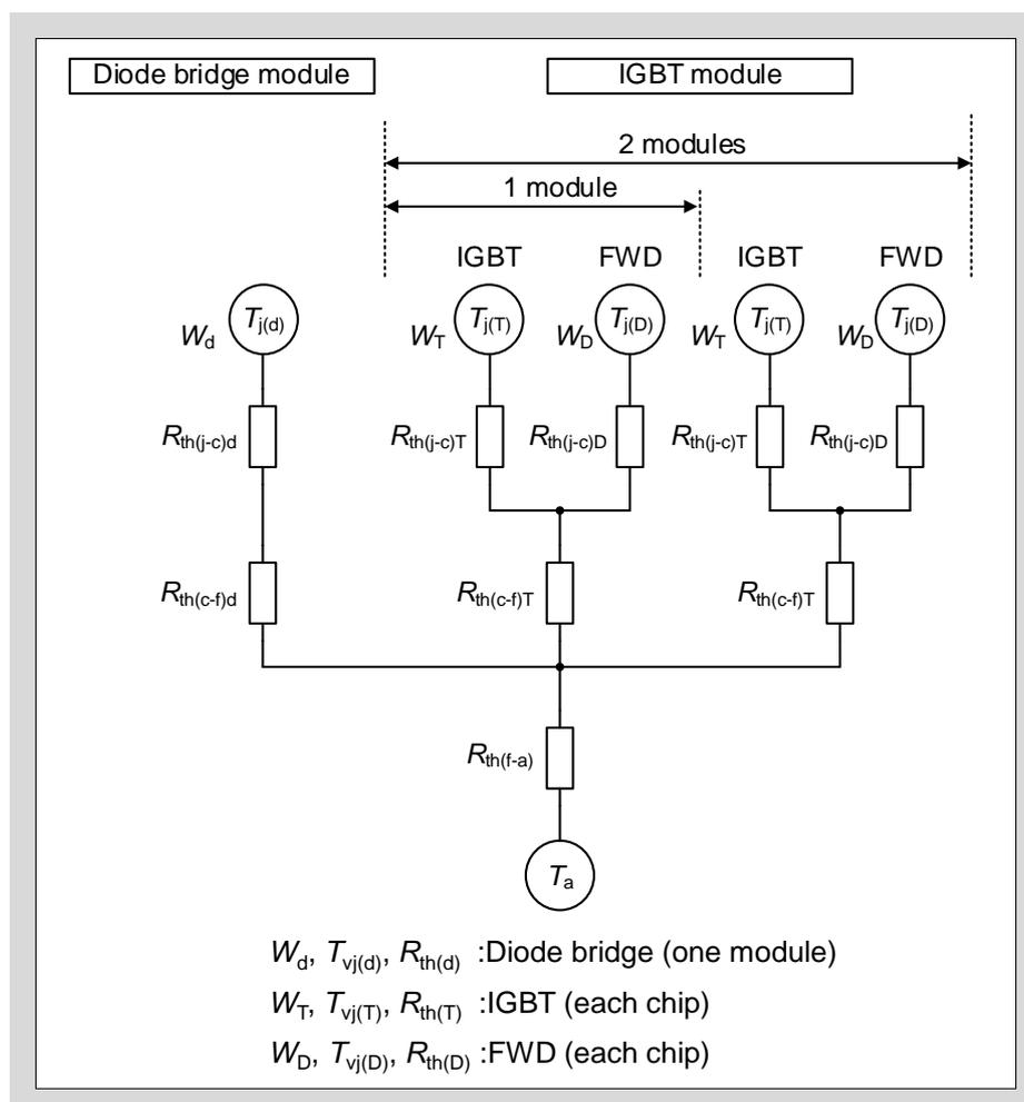
Fig. 6-10 Thermal resistance equivalent circuit
