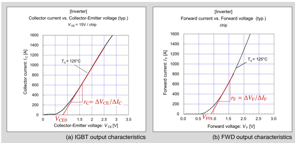
Fig. 6-5 Linear approximation of output characteristics
