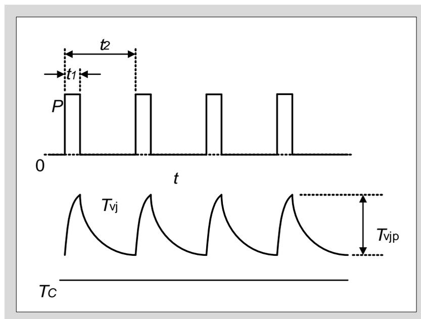
Fig. 6-12 Thermal ripples
