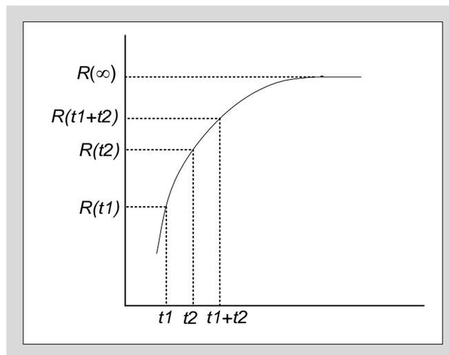
Fig. 6-11 Transient thermal resistance curve
