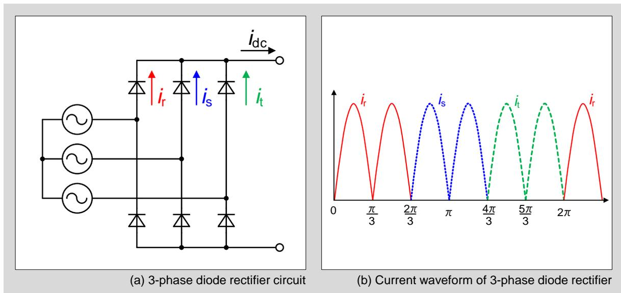
Fig. 6-7 3-phase diode rectifier circuit and current waveform
