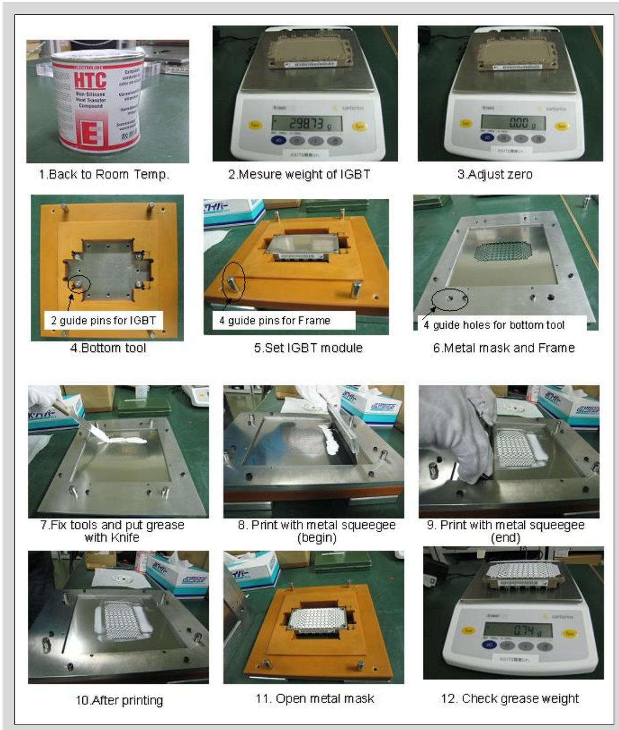
Fig. 6-13 Schematic diagram of example of thermal grease application
