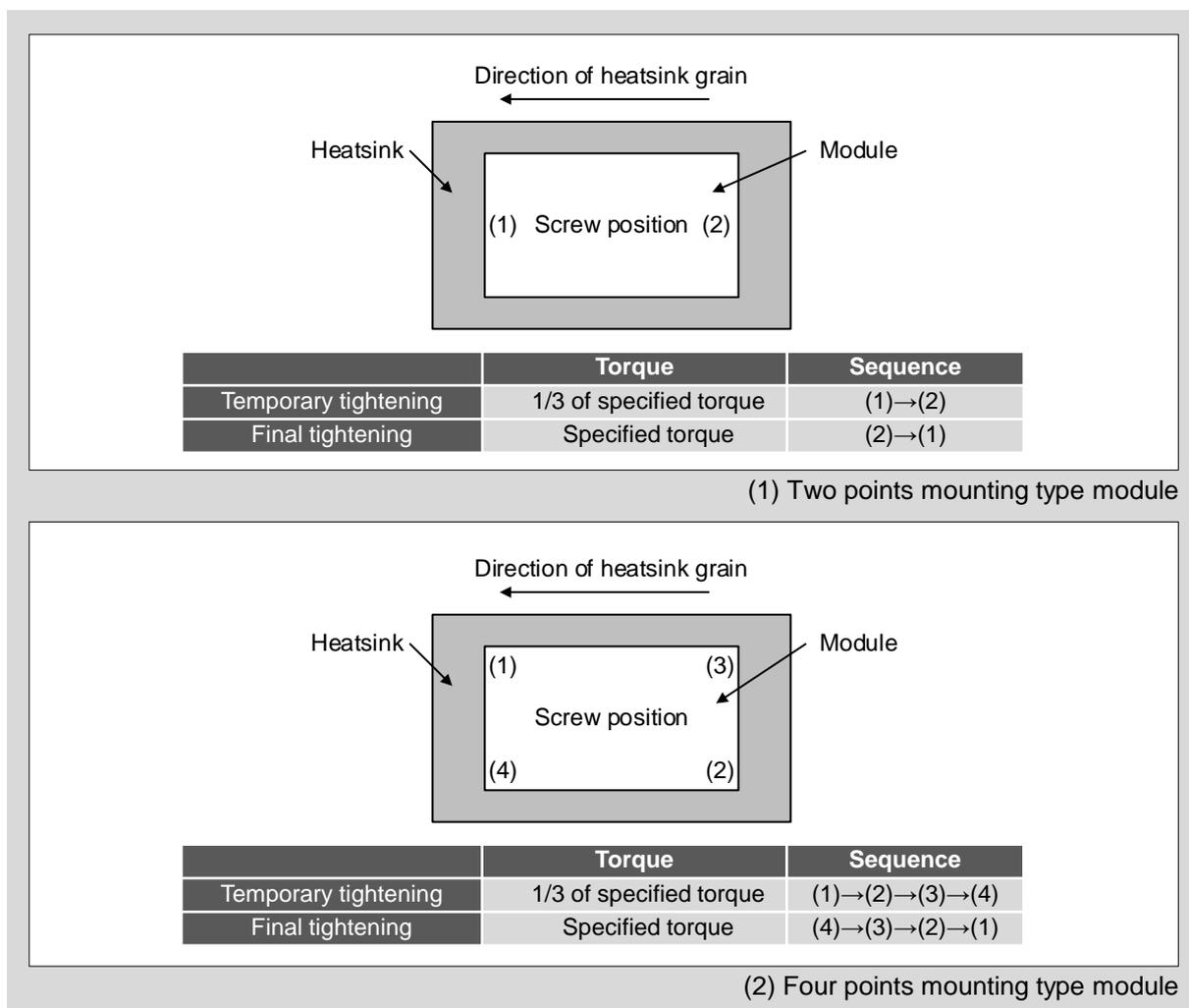
Fig. 6-14 Mounting procedure
