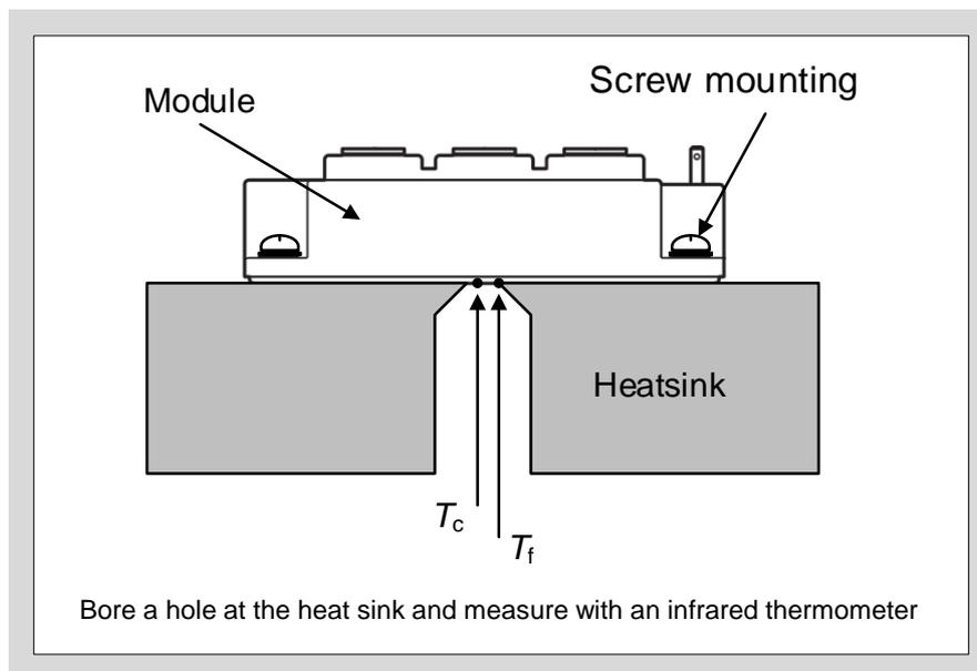
Fig. 6-15  $T_C$  measurement method
