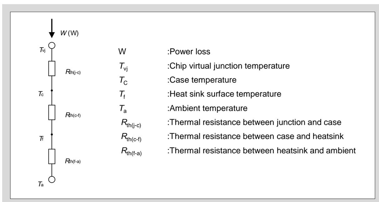
Fig. 6-8 Thermal resistance equivalent circuit
