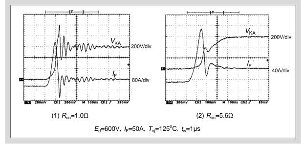
Fig. 4-9 shows the waveforms of short on-pulse reverse recovery of 6MBI450U-120 (1200V, 450A). As shown in the waveforms, surge voltage can be decreased by increasing  $R_{\rm G}$  from 1.0 $\Omega$  to 5.6 $\Omega$ .
