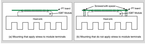
Fig. 4-5 Fixing a PCB
