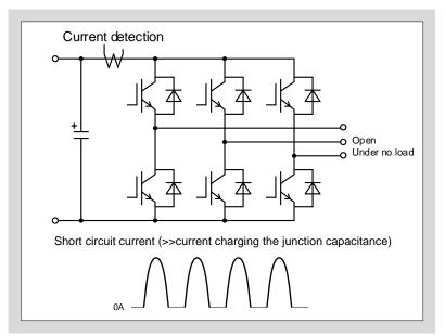
Fig. 4-7 Short circuit current measuring circuit
