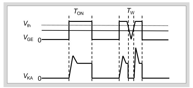
Fig. 4-8 Waveforms at short on-pulse reverse recovery
