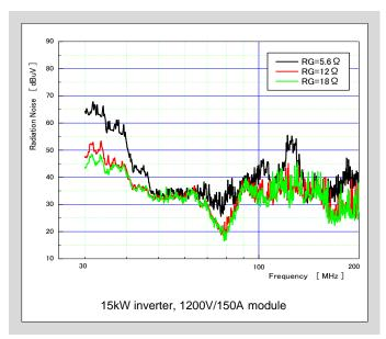
Fig. 4-11 Radiation noise ( $R_{G}$  dependence)
