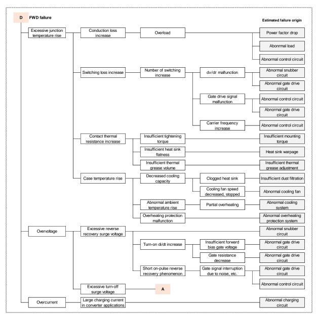
Fig. 4-1(e) Mode D: FWD failure
