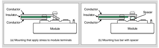
Fig. 4-6 Mounting with laminated bus bar
