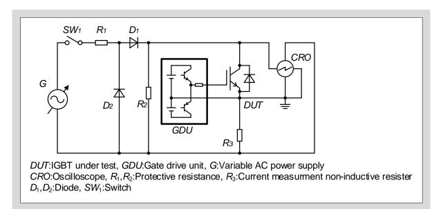
Fig. 4-4 On voltage measurement circuit
