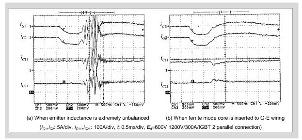
Fig. 4-10 Waveforms of 2 parallel connection
