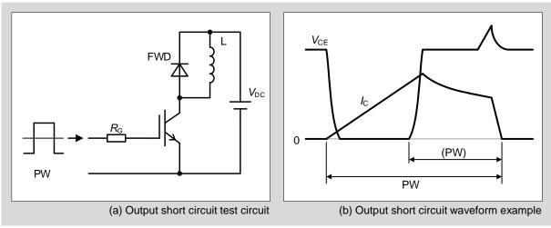
Fig. 5-2 Output short circuit test circuit and waveform
