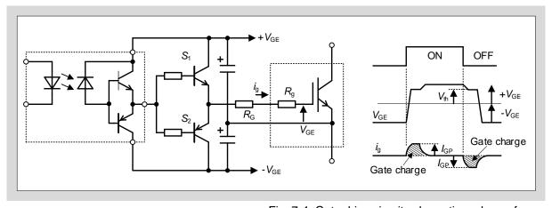
Fig. 7-4 Gate drive circuit schematic and waveforms
