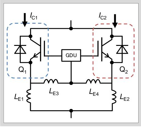
Fig. 8-8 Equivalent circuit of main circuit with wiring inductance component
