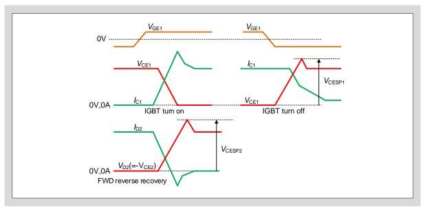
Fig. 5-7 Switching waveforms
