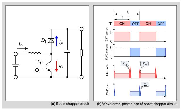
Fig. 6-3 Power loss in boost chopper circuit
