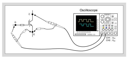
Fig. 9-10 Voltage probes connection
