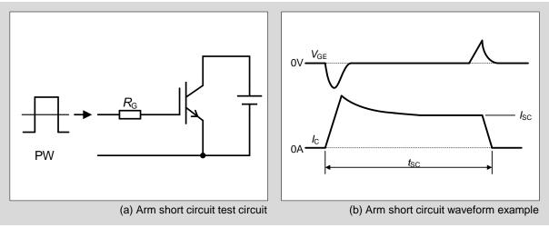
Fig. 5-1 Arm short circuit test circuit and waveform
