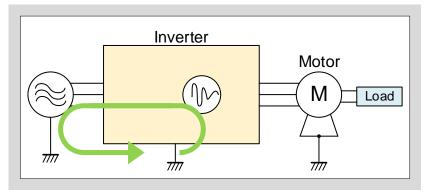
Fig. 10-6 Path of common mode noise
