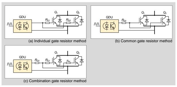
Fig. 8-13 Gate resistor configuration in common driver method
