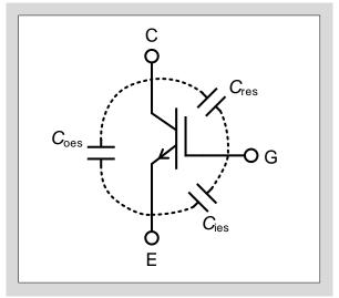
Fig. 2-13 Junction capacitance
