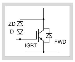
Fig. 5-12 Active clamp circuit
