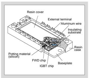
Fig. 1-3 Wire terminal connection structure type
