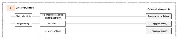
Fig. 4-1(c) Mode B: Gate overvoltage
