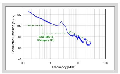
Fig. 10-13 Example of conducted emission of PDS
