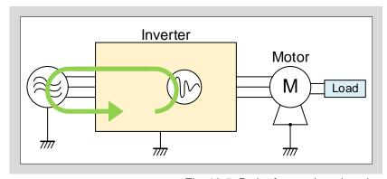
Fig. 10-5 Path of normal mode noise
