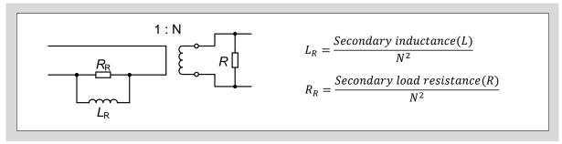
Fig. 9-11 Probe insertion impedance
