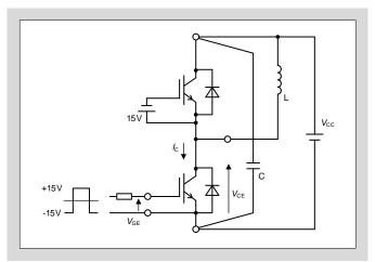
Fig. 2-4 Switching characteristics measuring circuit
