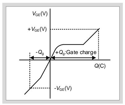
Fig. 7-3 Gate charge (Dynamic input) characteristics
