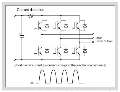
Fig. 4-7 Short circuit current measuring circuit
