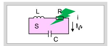
Fig. 10-26 Loop composed of IGBT module and snubber C
