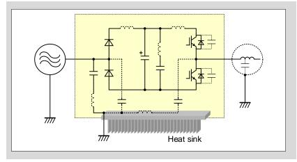
Fig. 10-10 Equivalent circuit considering stray L and C
