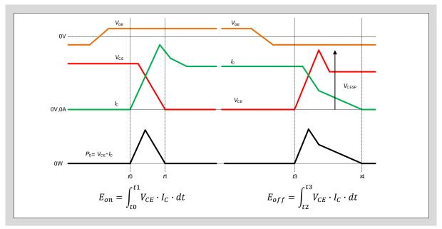
Fig. 9-5 Switching loss
