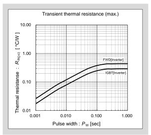
Fig. 2-17 Transient thermal resistance
