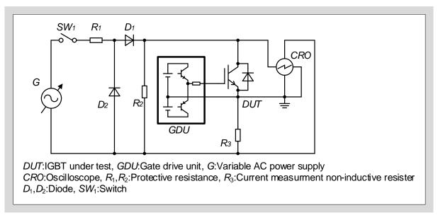
Fig. 4-4 On voltage measurement circuit
