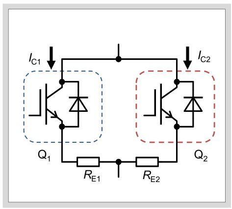
Fig. 8-7 Equivalent circuit of main circuit with wiring resistance component
