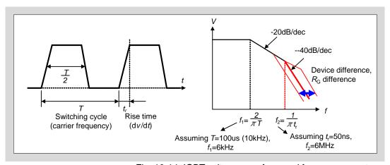
Fig. 10-14 IGBT voltage waveform and frequency spectrum
