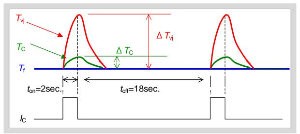
Fig. 11-2  $\Delta T_{vi}$ -P/C test current pattern and temperature changes
