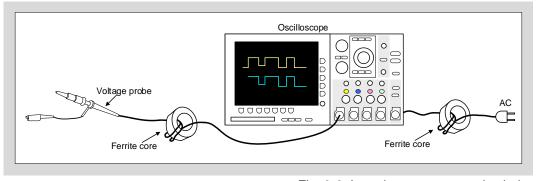
Fig. 9-6 Inserting common mode choke
