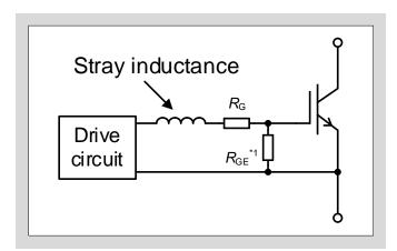
Fig. 7-8 Precautions for gate drive circuit design
