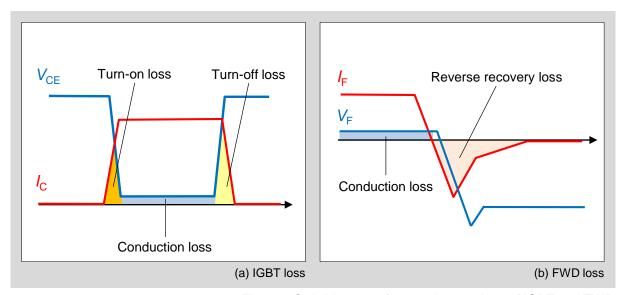
Fig. 6-1 Switching waveform and power loss of IGBT and FWD
