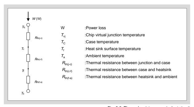
Fig. 6-8 Thermal resistance equivalent circuit
