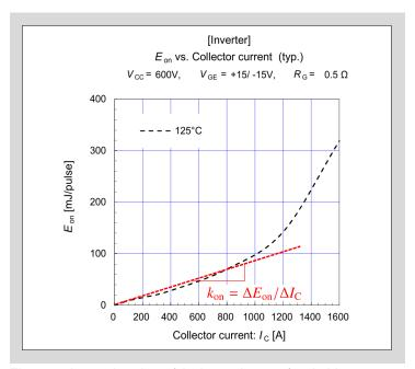
Fig. 6-6 Approximation of  $I_{\mathbb{C}}$  dependence of switching energy
