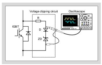
Fig. 9-1 Measurement method of saturation voltage
