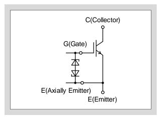
Fig. 7-9 G-E overvoltage protection circuit example
