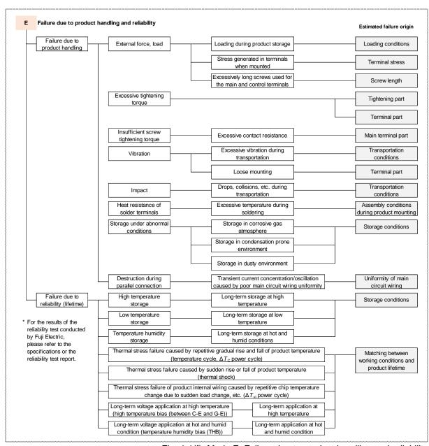
Fig. 4-1(f) Mode E: Failure due to product handling and reliability
