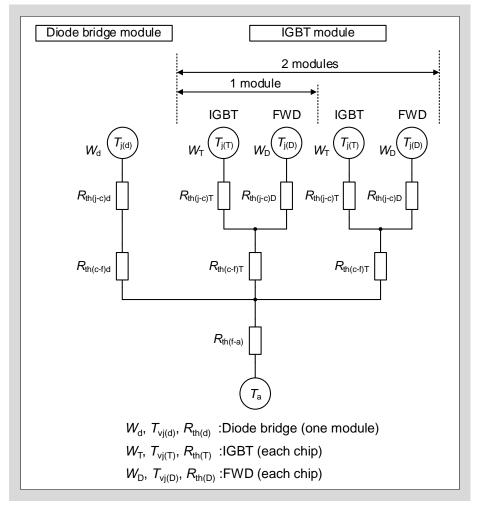
Fig. 6-10 Thermal resistance equivalent circuit
