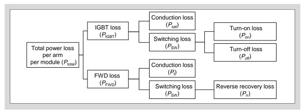
Fig. 6-2 Classification of IGBT module power loss
