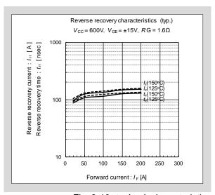
Fig. 2-16  $t_{rr}$ ,  $I_{rr}$  -  $I_{F}$  characteristics
