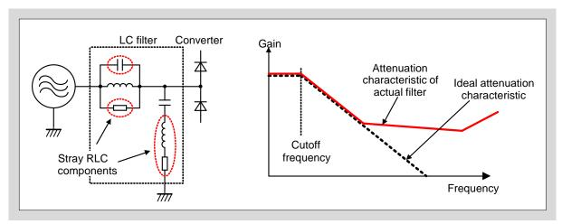
Fig. 10-17 Attenuation characteristics of ideal filter and actual filter
