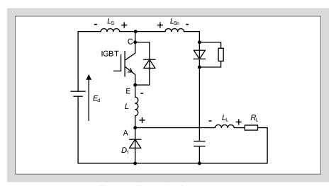
Fig. 9-2 Example of surge voltage measurement circuit
