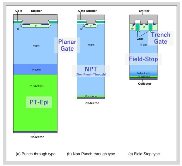
Fig. 1-1 Structure comparison of IGBT
