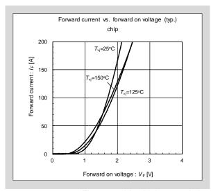
Fig. 2-15  $V_F$  -  $I_F$  characteristics
