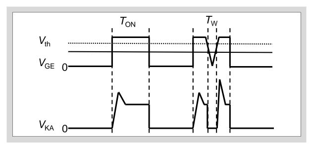
Fig. 4-8 Waveforms at short on-pulse reverse recovery
