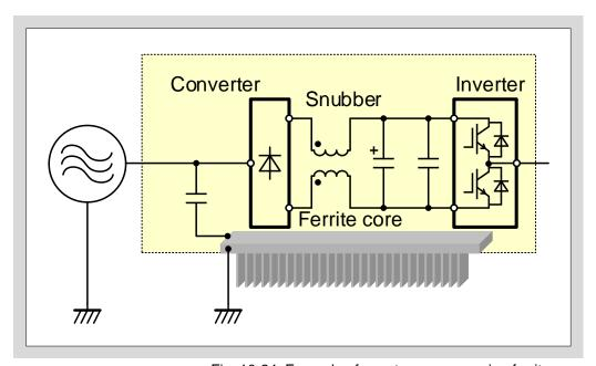
Fig. 10-24 Example of countermeasure using ferrite core
