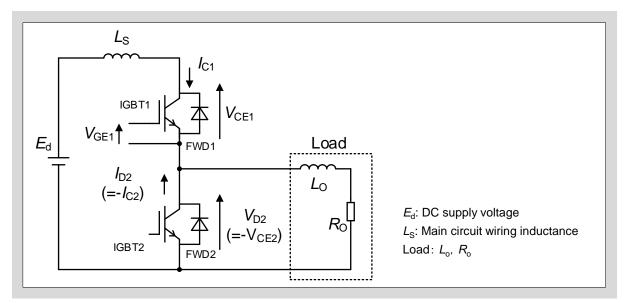
Fig. 5-6 Chopper circuit
