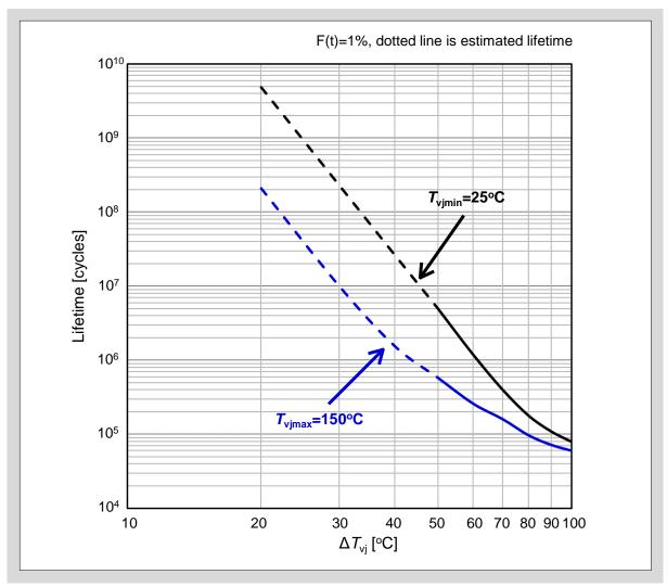
Fig. 11-5 Example of  $\Delta T_{vi}$ -P/C lifetime curve
