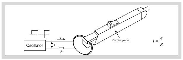
Fig. 9-3 Current probe calibration method
