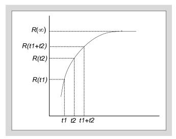
Fig. 6-11 Transient thermal resistance curve
