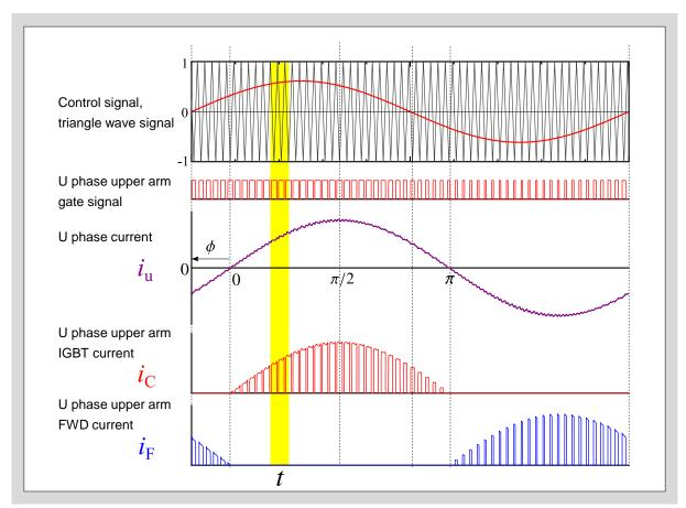
Fig. 6-4 Operating waveform of a 3-phase 2-level PWM inverter
