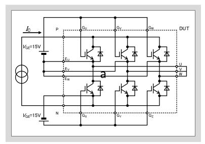
Fig. 11-8 Equivalent test circuit for  $\Delta T_{\rm C}$ -P/C test
