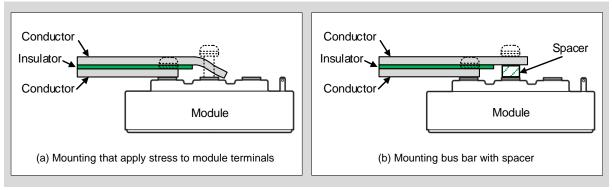
Fig. 4-6 Mounting with laminated bus bar
