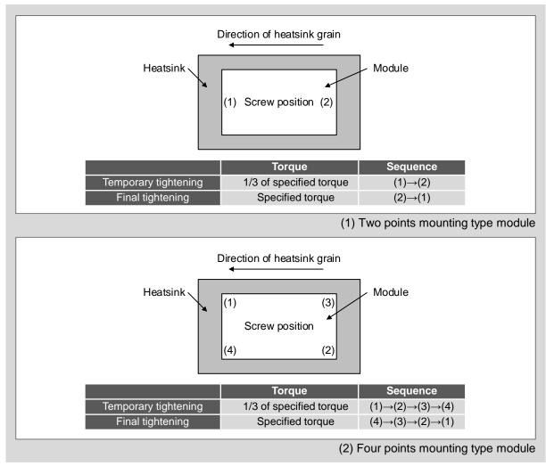
Fig. 6-14 Mounting procedure
