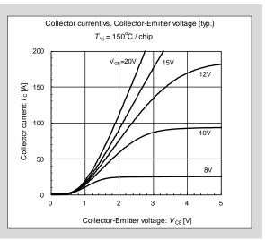
Fig. 2-2  $V_{CE(sat)}$  -  $I_C$  characteristics ( $T_{vi}$ =150 $^{\circ}$ C)
