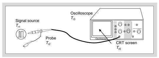
Fig. 9-8 Measurement system and rise time of each component
