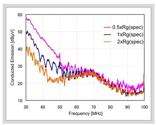
Fig. 10-28 Radiated emission dependence on gate resistance (7MBR100U4B-120)
