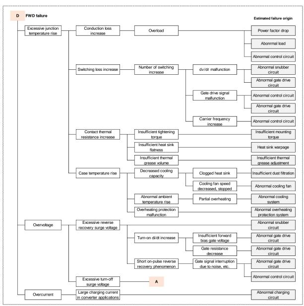
Fig. 4-1(e) Mode D: FWD failure
