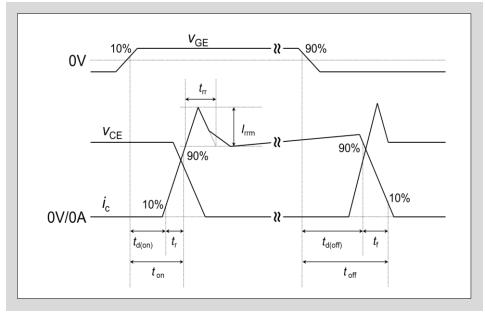
Fig. 2-5 Definition of switching time
