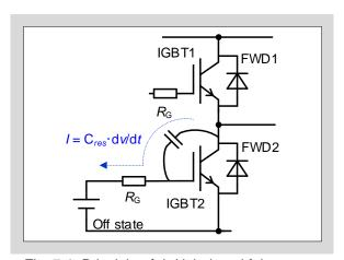
Fig. 7-1 Principle of dv/dt induced false turn-on
