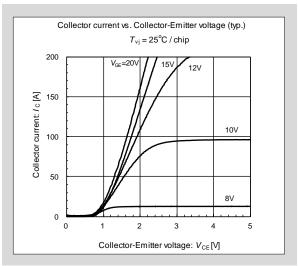
Fig. 2-1  $V_{CE(sat)}$  -  $I_C$  characteristics ( $T_{vi}$ =25°C)
