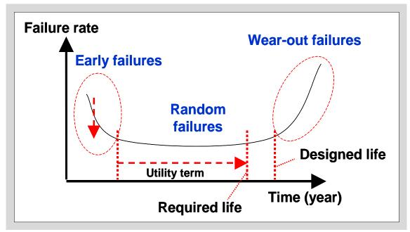
Fig. 11-1 Change in failure rate of semiconductor devices over time
