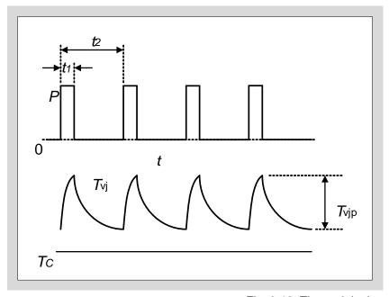
Fig. 6-12 Thermal ripples
