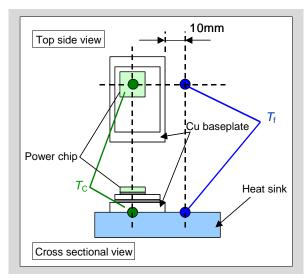
Fig. 11-4  $T_C$  and  $T_f$  measurement positions
