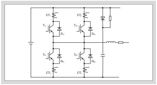
Fig. 9-4 CT insert position and current measurement method
