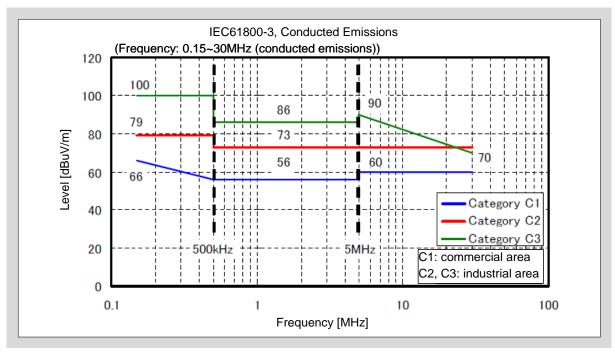
Fig. 10-2 Limits of conducted emissions in IEC61800-3
