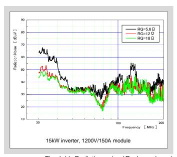
Fig. 4-11 Radiation noise ( $R_G$  dependence)
