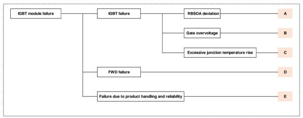
Fig. 4-1(a) IGBT module failure analysis chart (\* Symbols A to D are linked to the charts below)
