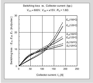
Fig. 2-9 Switching loss - I<sub>C</sub> characteristics
