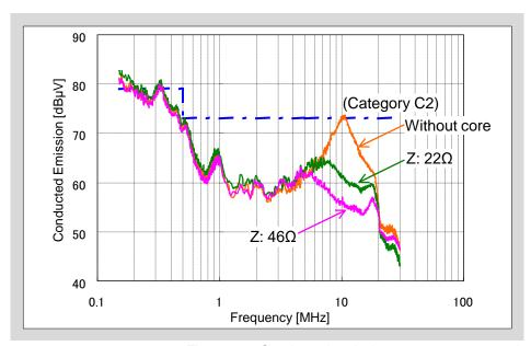
Fig. 10-25 Conducted emission measurement result
