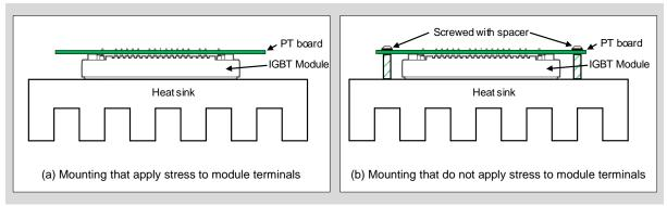
Fig. 4-5 Fixing a PCB
