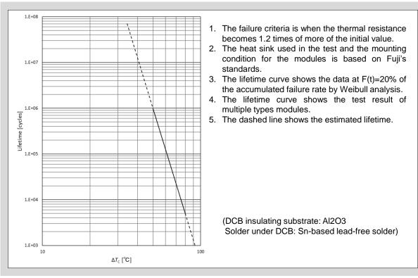
Fig. 11-9 Example of  $\Delta T_{\rm C}$ -PC lifetime
