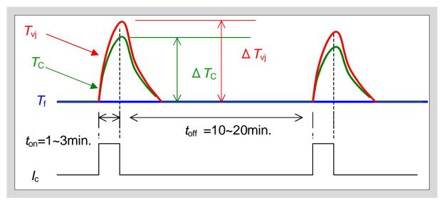
Fig. 11-7  $\Delta T_{\rm C}$ -P/C test current pattern and temperature changes
