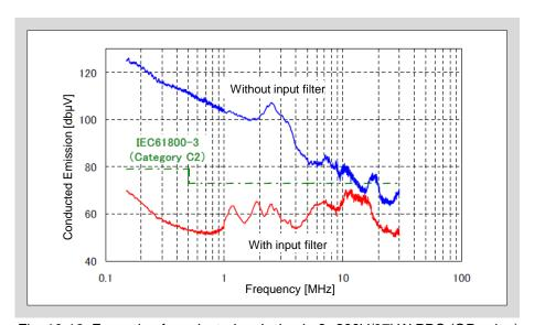
Fig. 10-16 Example of conducted emission in 3φ200V/37kW PDS (QP value)
