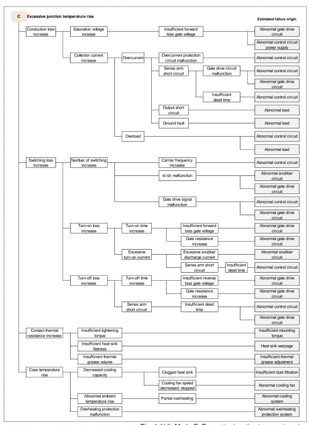
Fig. 4-1(d) Mode C: Excessive junction temperature rise
