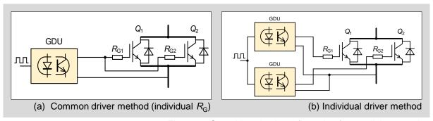
Fig. 8-11 Gate drive circuit configuration for parallel connection
