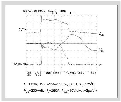
Fig. 5-5 Waveforms during short circuit protection
