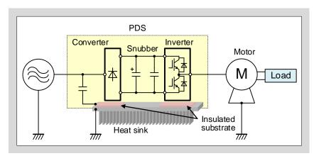
Fig. 10-9 Example of power drive system
