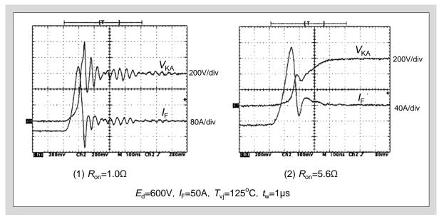
Fig. 4-9 Waveforms of short on-pulse reverse recovery
