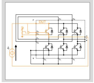
Fig. 11-3 Equivalent test circuit for  $\Delta T_{vi}$ -PC test
