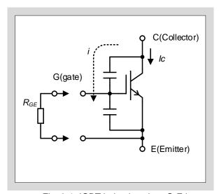
Fig. 3-1 IGBT behavior when G-E is open
