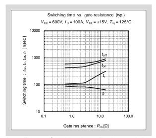
Fig. 2-8 Switching time -  $R_G$  characteristics ( $T_{vi}$ =125°C)
