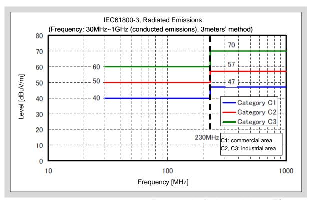
Fig. 10-3 Limits of radiated emissions in IEC61800-3
