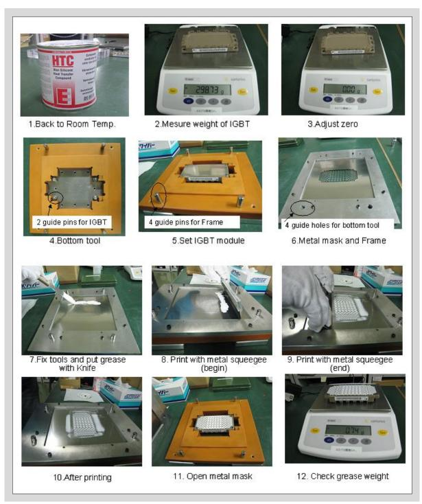
Fig. 6-13 Schematic diagram of example of thermal grease application
