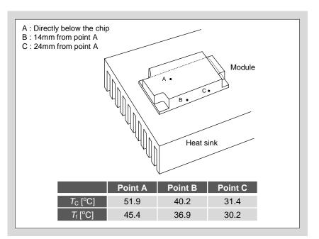
Fig. 6-9 Example of case and heatsink temperature measurement
