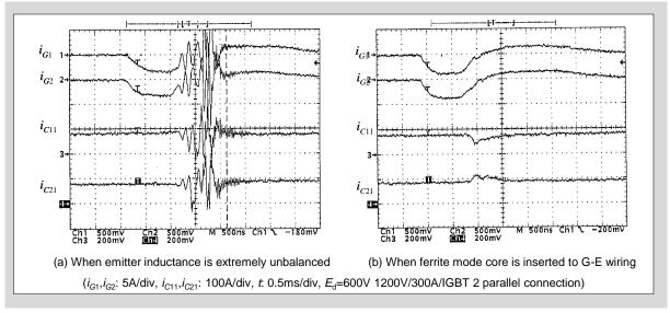
Fig. 4-10 Waveforms of 2 parallel connection
