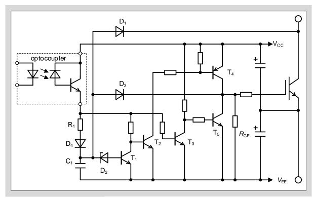
Fig. 5-4 Short-circuit protection circuit using  $V_{\mathrm{CE(sat)}}$  detection method
