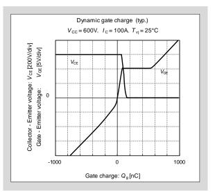
Fig. 2-11  $V_{CE}$ ,  $V_{GE}$  -  $Q_g$  characteristics
