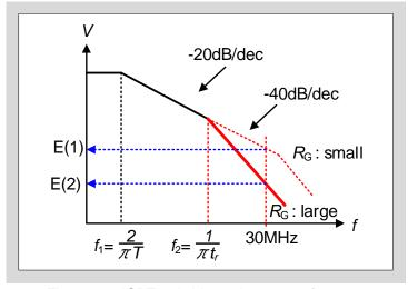
Fig. 10-27 IGBT switching voltage waveform spectrum
