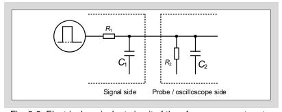
Fig. 9-9 Electrical equivalent circuit of the of measurement system
