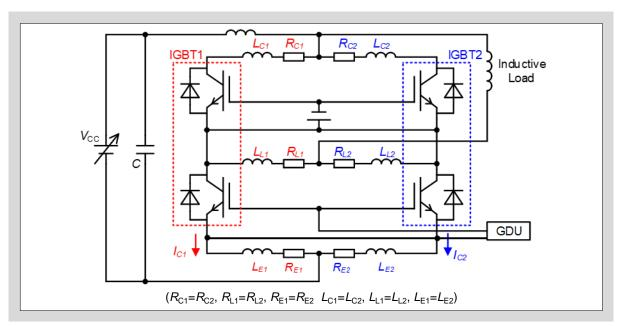
Fig. 8-9 Equivalent circuit when paralleling two 2-Pack modules
