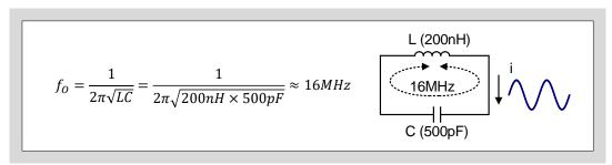
Fig. 10-11 Resonance phenomenon between stray inductance and stray capacitance
