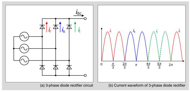
Fig. 6-7 3-phase diode rectifier circuit and current waveform
