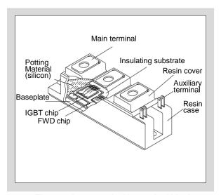
Fig. 1-2 Integrated with terminal block type
