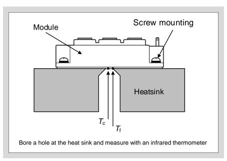
Fig. 6-15  $T_{\rm C}$  measurement method
