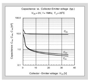
Fig. 2-12 Junction capacitance characteristic
