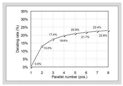
Fig. 8-6 Relationship between derating rate and parallel number
