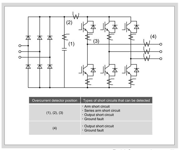
Fig. 5-3 Overcurrent detector position
