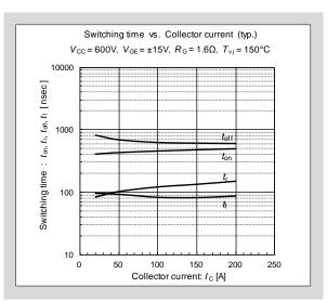
Fig. 2-7 Switching time -  $I_C$  characteristics  $(T_{vi}=150^{\circ}C)$
