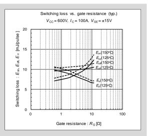
Fig. 2-10 Switching loss - R<sub>G</sub> characteristics
