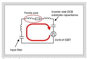
Fig.10-22 Equivalent circuit when ferrite core is inserted
