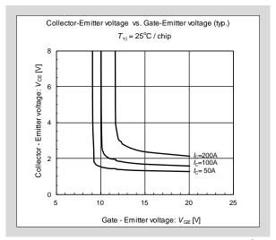
Fig. 2-3  $V_{CE}$  -  $V_{GE}$  characteristics ( $T_{vi}$ =25°C)
