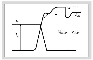
Fig. 5-10 Turn-off waveform with discharge-suppressing RCD snubber circuit
