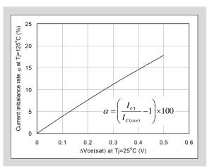
Fig. 8-1 Example of different output characteristics
