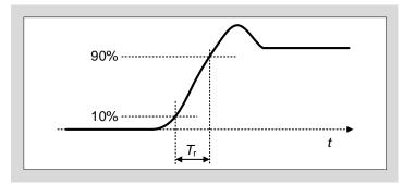
Fig. 9-7 Definition of the rise time of pulse waveform
