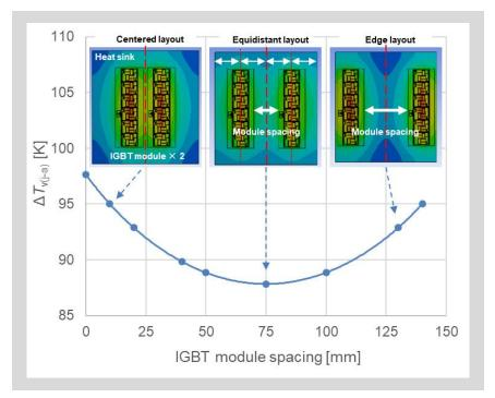
Fig. 8-14  $\Delta T_{v(i-a)}$ -IGBT module spacing dependency
