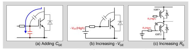
Fig. 7-2 Countermeasures against dv/dt induced false turn-on
