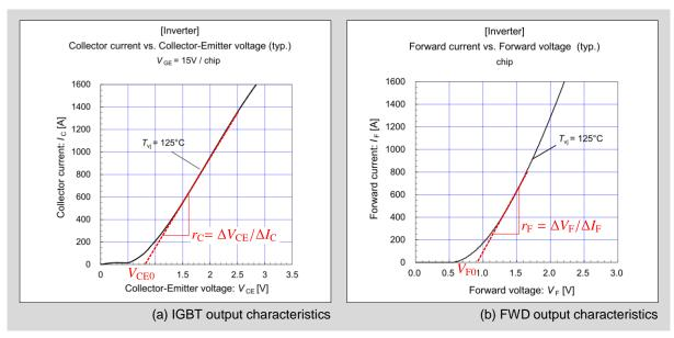
Fig. 6-5 Linear approximation of output characteristics
