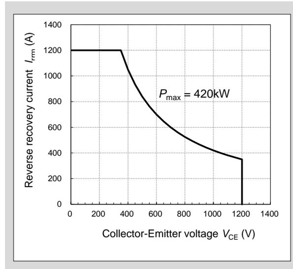
Fig.2-9 Example of Safe Operating Area (SOA) for FWD
