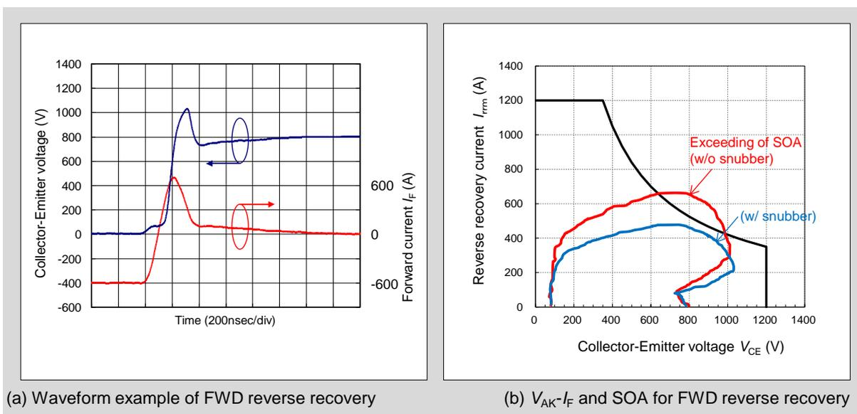
Fig.2-10 Reverse recovery waveform and  $V_{AK}$ - $I_F$  locus for FWD reverse recovery
