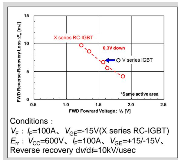
Fig.3-6 Trade-off relationship of X series RC-IGBT (FWD)
