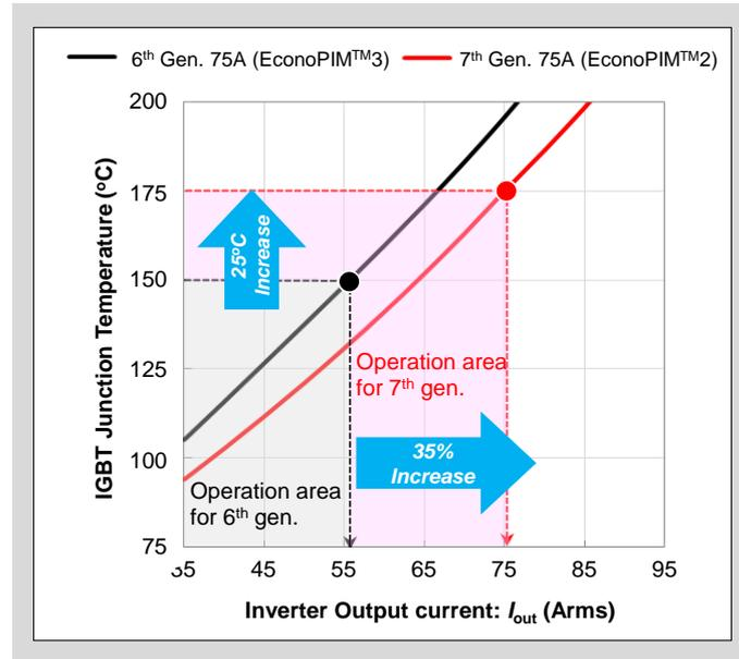
Fig.1-13 Inverter output current vs. junction temperature
