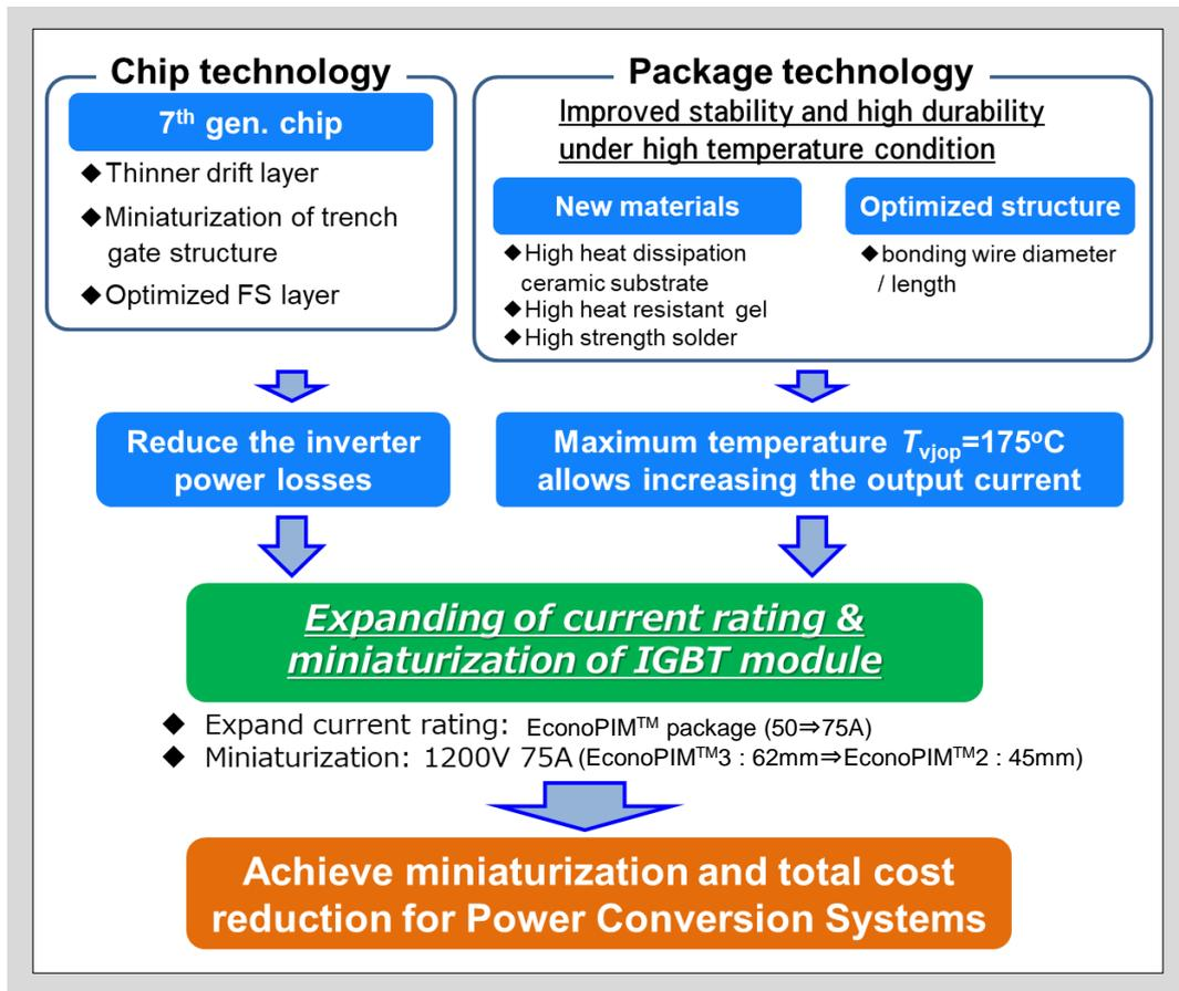
Fig.1-1 The basic concept of 7<sup>th</sup> generation X-series IGBT modules
