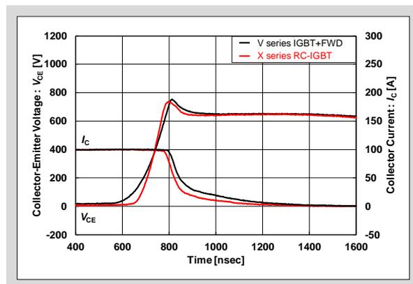
Fig.3-3 Turn off waveform of X series RC-IGBT
