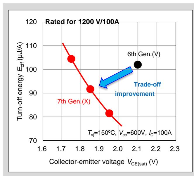
Fig.1-5 Improvement of turn-off energy vs. on-state voltage
