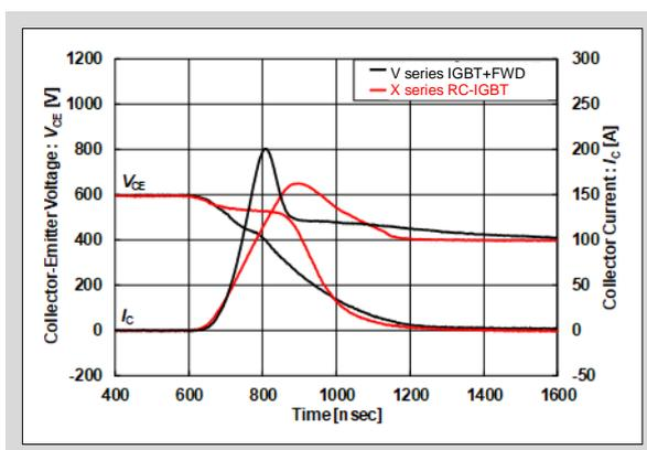
Fig.3-4 Turn on waveform of X series RC-IGBT
