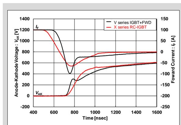
Fig.3-5 Reverse recovery waveform of X series RC-IGBT
