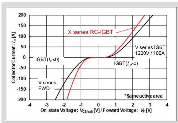
Fig.3-2 Output characteristics of X series RC-IGBT
