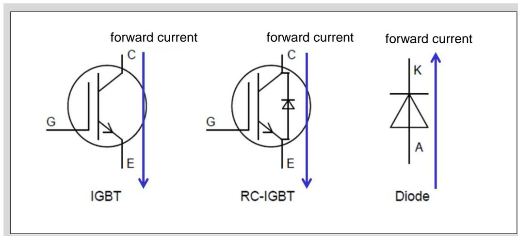
Fig.1-15 Definition of forward current
