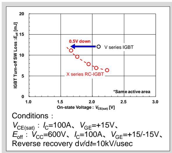
Fig.3-6 Trade-off relationship of X series RC-IGBT (IGBT)
