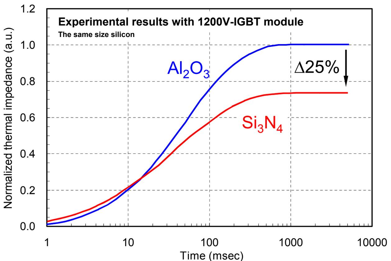
Fig. 4-1 Comparison of Transient Thermal Impedance Characteristics
