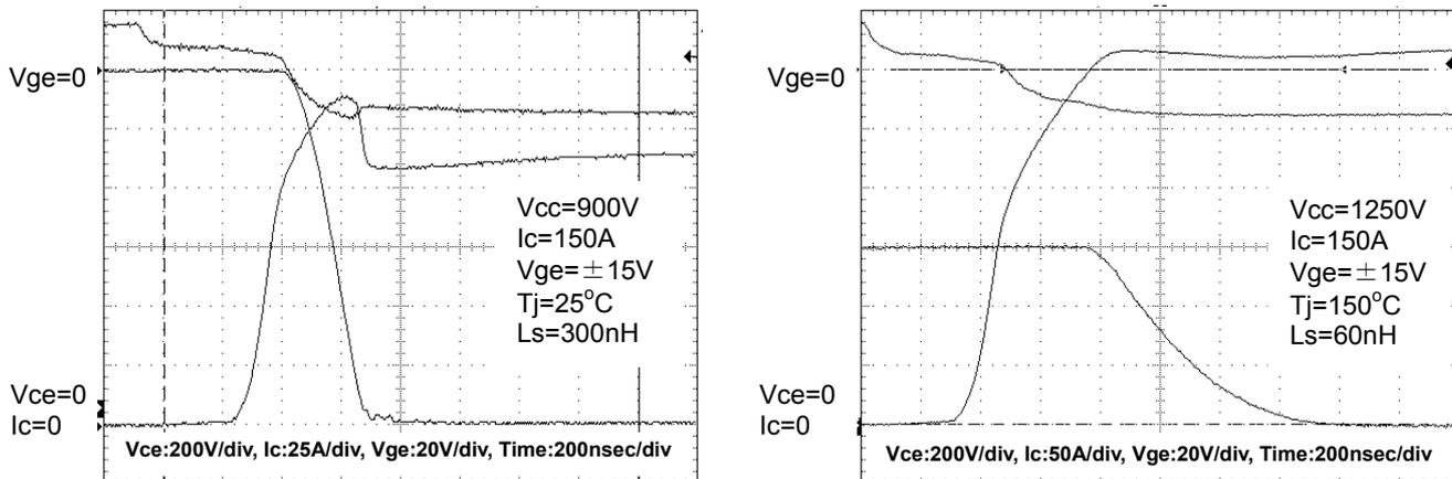
Fig. 3-3 Turn-off Waveforms of V-IGBT (75A / 1200V)
