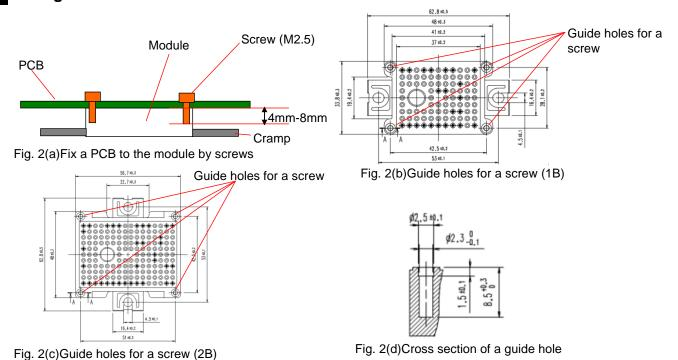
After soldering process, it is recommended to fix a PCB to the module by screws because of the solder joint reliability. Fig. 2(a) shows an example of fixing process. M2.5 screws are suitable. The effective length of a screw except the PCB thickness, have to be 4.0-8.0mm. Screwdriver speed n must be smaller than 300rpm, screw driver torque; 0.4Nm±10% s recommended.
