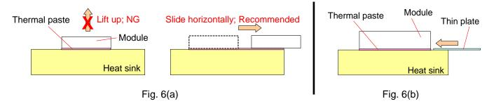
Fig. 6 An example of removal process after the screwing
