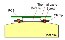
Fig. 3(b) Flatness of a heat sink
