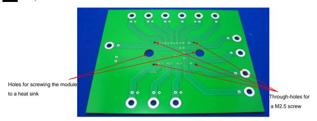
Fig. 1 An example of a PCB
