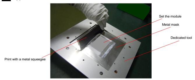
Fig. 4 Stencil printing process
