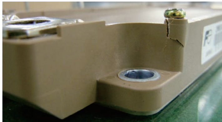
Fig.7 Example of damaged module by wrong screw
