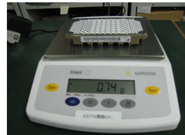
12. Check grease weight
