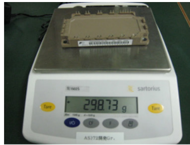
2. Measure weight of IGBT
