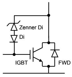
Fig. 5-11 Active clamp circuit
