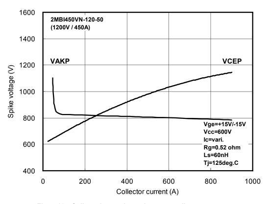
Fig. 5-10 Spike voltages dependency on collector current
