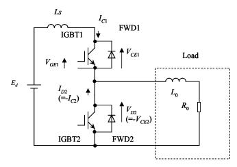
E<sub>d</sub>: DC supply voltage, L<sub>S</sub>: Main circuit wiring inductance, Load:L<sub>0</sub>,R<sub>0</sub>
