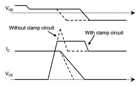
Fig. 5-12 Schematic waveform for active clamp circuit
