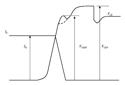
Fig. 5-9 Voltage and current waveforms at turn-off
