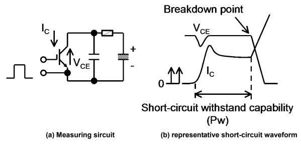
Fig. 5-1 Measuring circuit and waveform
