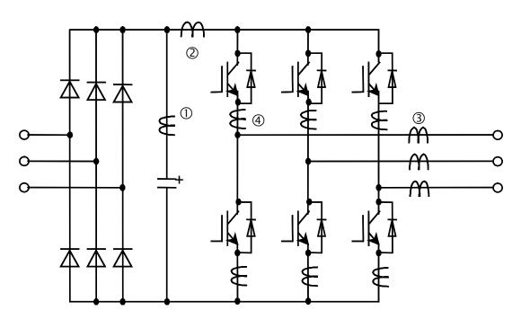
Fig. 5-2 Overcurrent detector insertion methods
