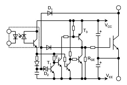
Fig. 5-3 Short-circuit protection schematic based in VCE(sat) detection
