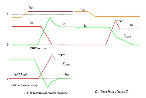
Fig. 5-6 Switching waveforms
