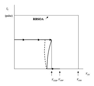
Fig. 5-8 Turn-off locus waveform of IGBT
