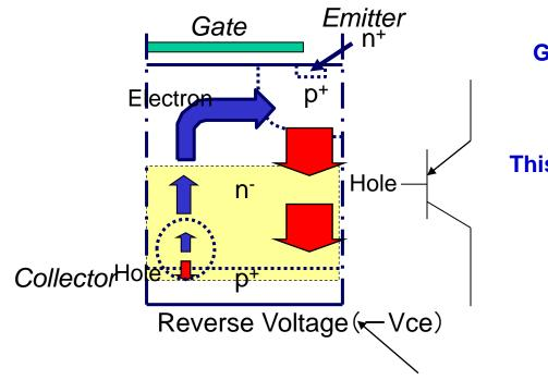
Generation of hole at Reverse voltage area ↓ Electron flow through the emitter area ↓ This electron is base current of PNP transistor Generation of Hole at P-layer ↓ Generation of Large leakage current
