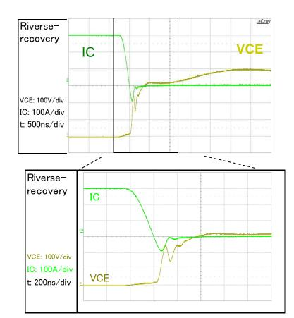
Fuji RB-IGBT can be realized of fast switching operation same as normal IGBT and FWD.
