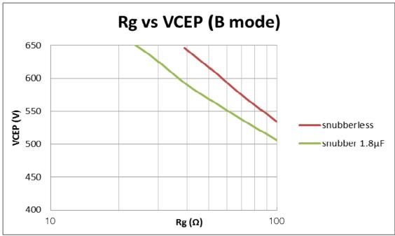
Dependence of spike voltage on gate resistance by the effect of snubber
