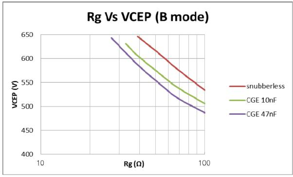
Dependence of spike voltage on gate resistance by the effect of CGE
