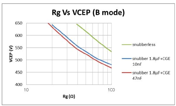
Dependence of spike voltage on gate resistance by the effect of snubber and CGE
