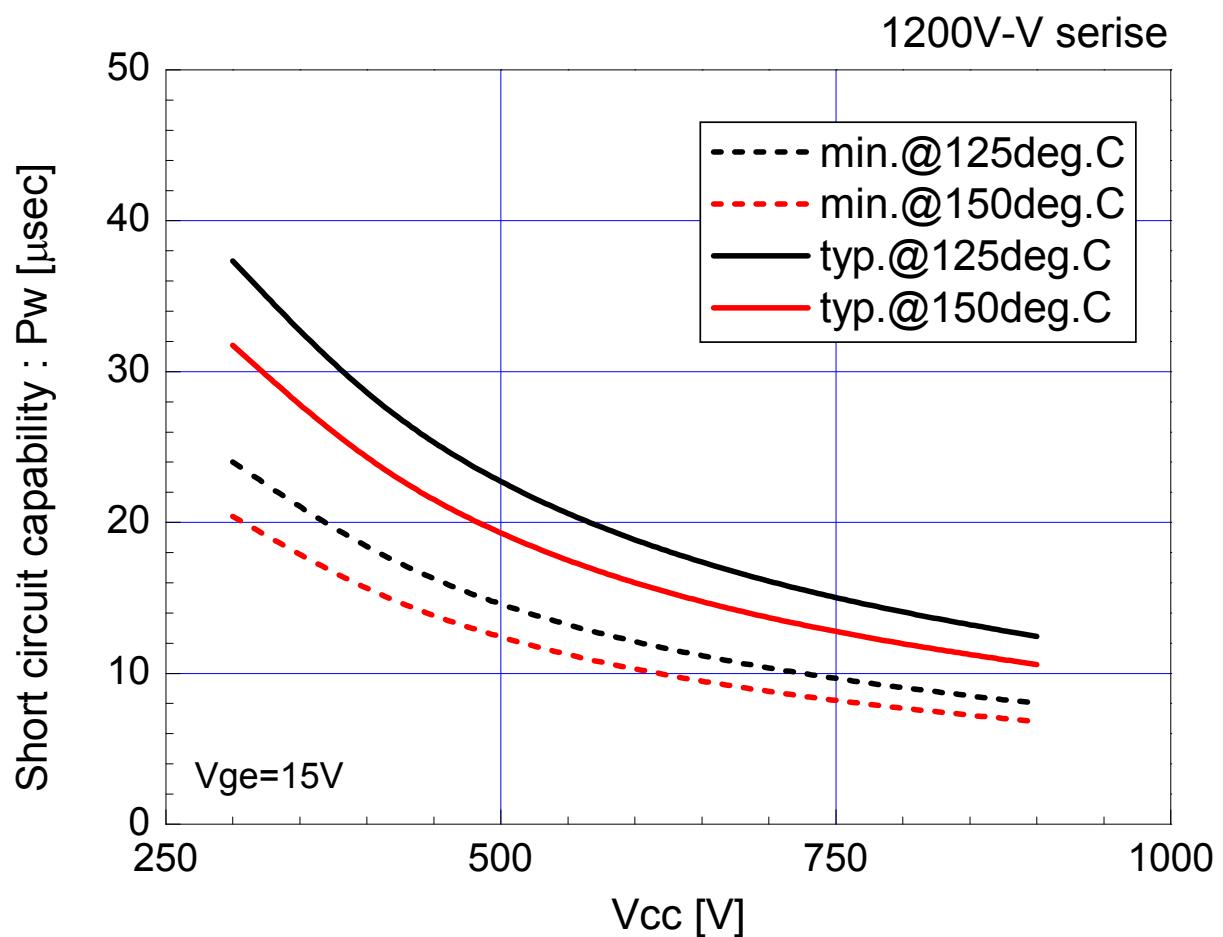
Fig. Relation between applied voltage and short-circuit capacity (1200V Family)
