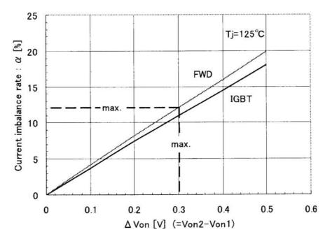
The rank division of  $V_{on}$  is unnecessary for U4 Series by the set value of  $\alpha$ =12% (IGBT:  $\alpha$ =11%, FWD:  $\alpha$ =12%). When connecting parallel the chips of N piece, overall permissible current is shown by the follow (I<sub>max</sub> is made maximum permissible current).
