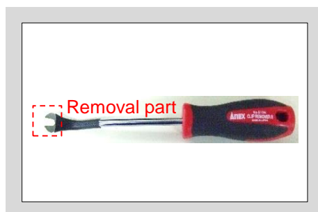
Fig. 2-2 Example of remover (removal jig)
