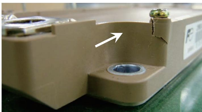
Fig.10 Mechanical damage example of IGBT module
