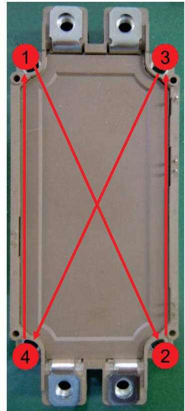
Fig.12 Mounting holes (1) ~ (4) in Press Fit module
