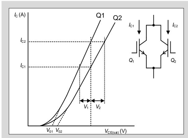
Fig. 8-1 Example of different output characteristics
