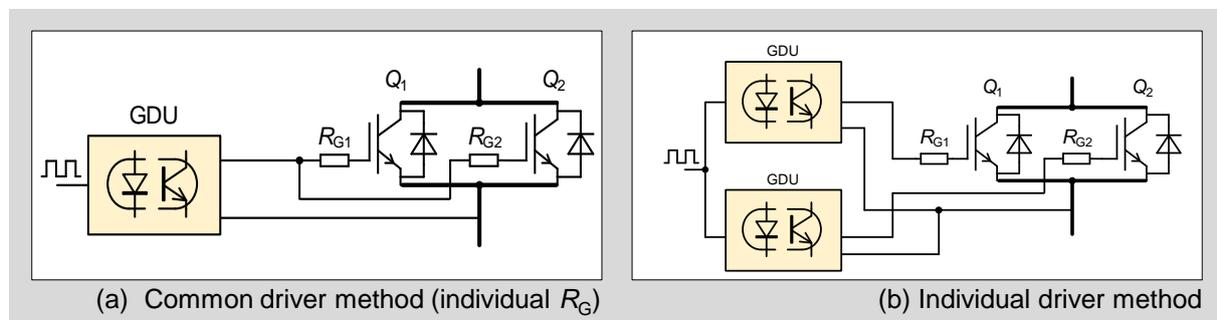
Fig. 8-11 Gate drive circuit configuration for parallel connection
