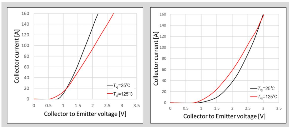
Fig. 8-5 Comparison of IGBT output characteristics (left: positive  $T_{vj}$  dependency, right: negative  $T_{vj}$  dependency)
