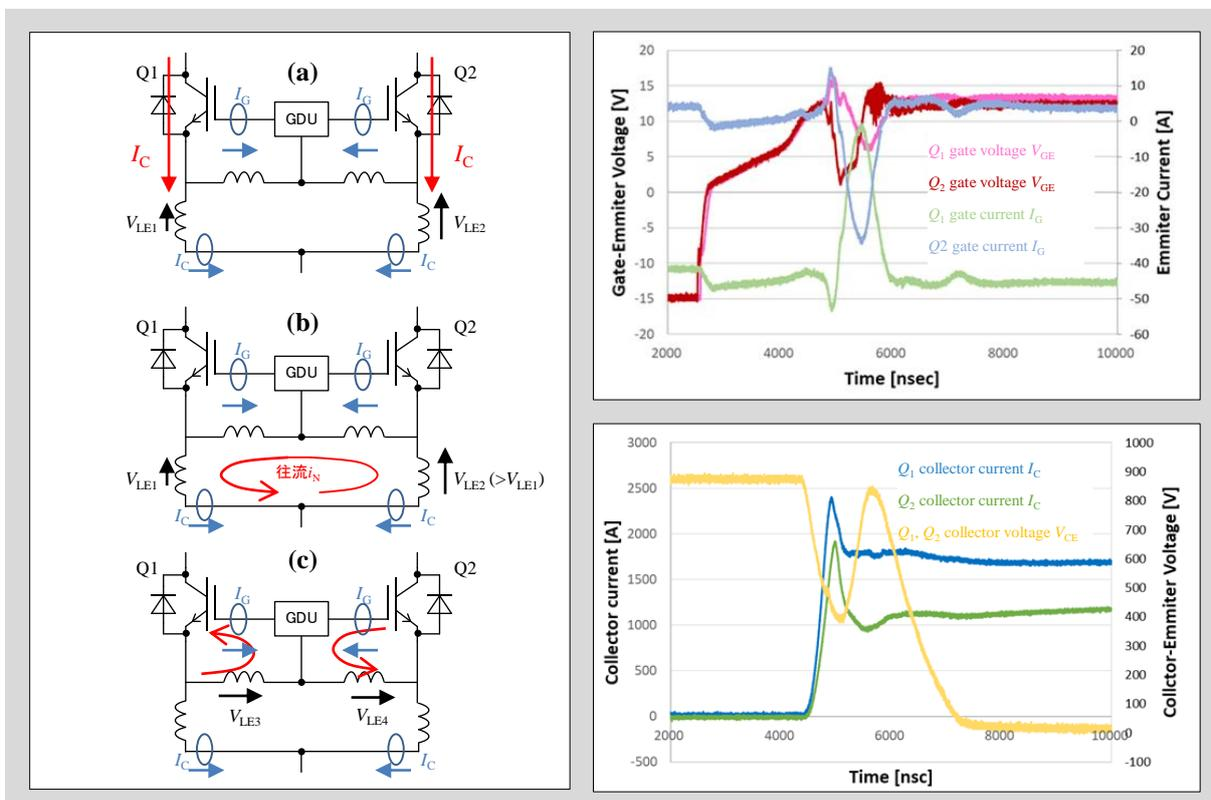
Fig. 8-12 Parasitic oscillation mechanism and turn-on waveforms
