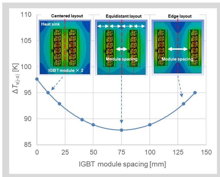
Fig. 8-14  $\Delta T_{v(j-a)}$ -IGBT module spacing dependency
