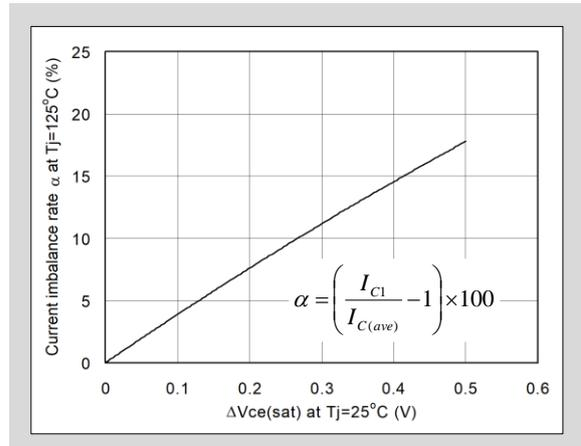
Fig. 8-2  $\Delta V_{CE(sat)}$  and current imbalance rate
