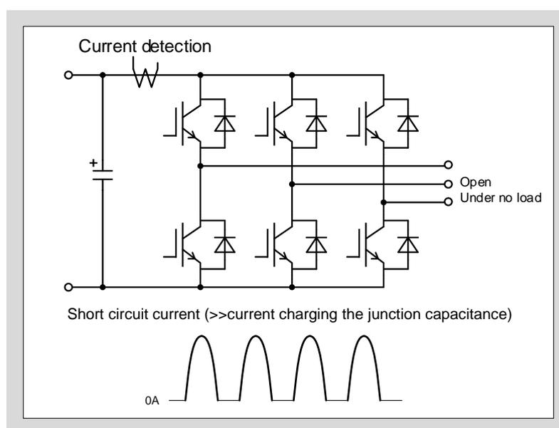
Fig. 4-7 Short circuit current measuring circuit
