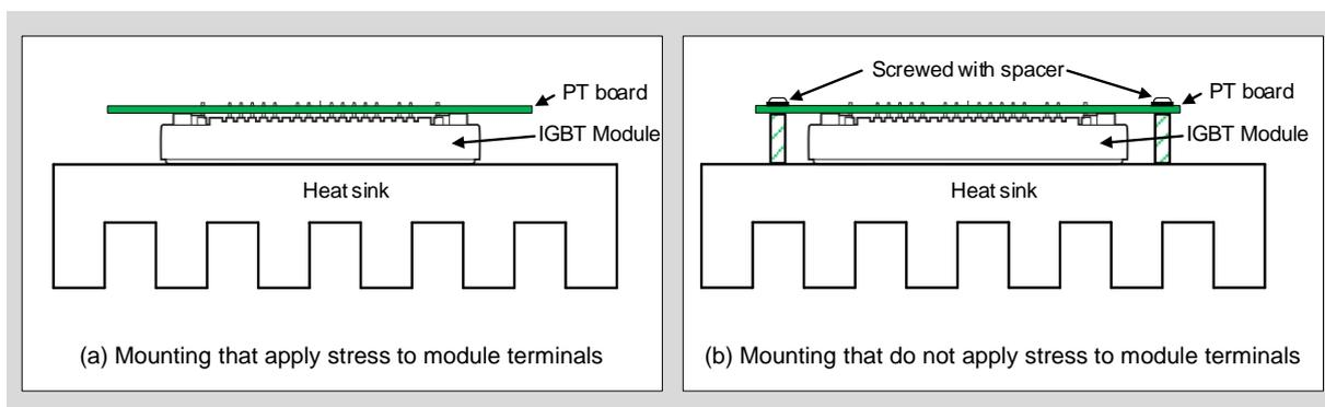
Fig. 4-5 Fixing a PCB
