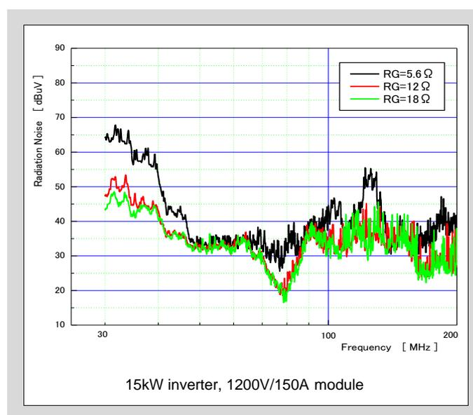
Fig. 4-11 Radiation noise ( $R_G$  dependence)
