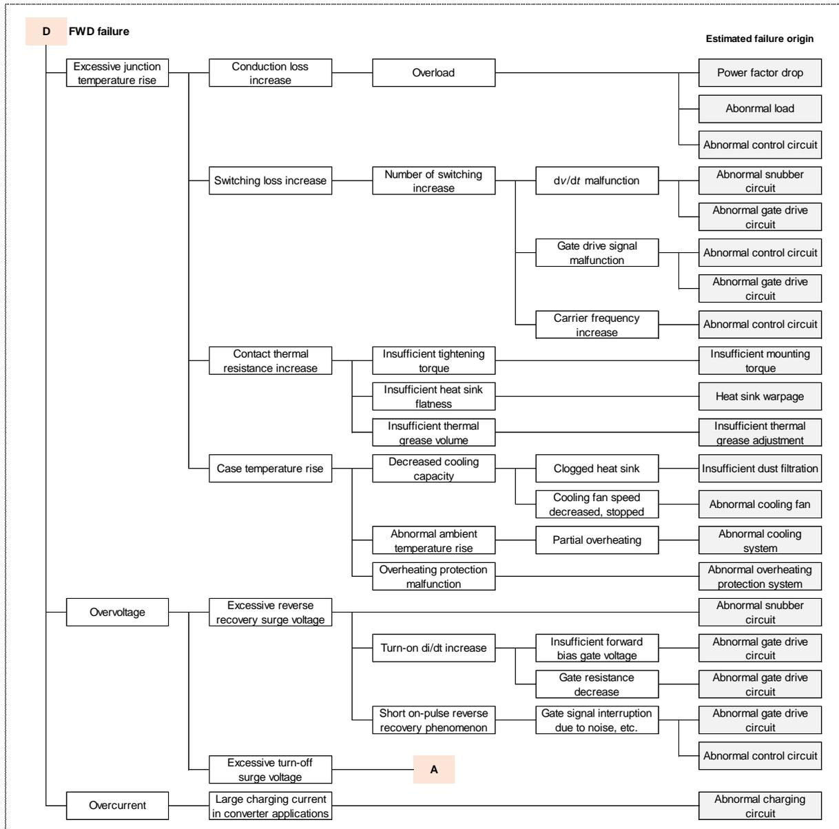
Fig. 4-1(e) Mode D: FWD failure
