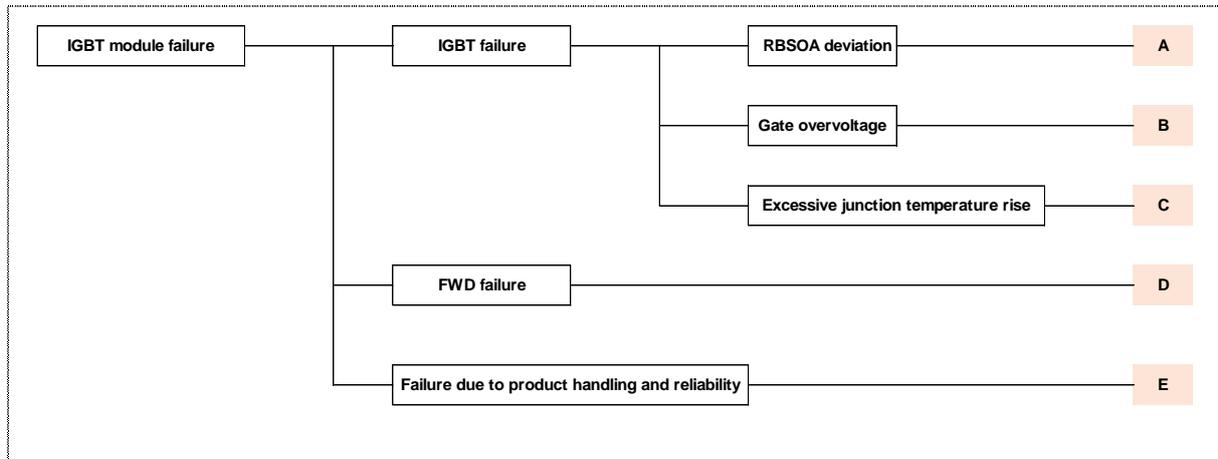
Fig. 4-1(a) IGBT module failure analysis chart (\* Symbols A to D are linked to the charts below)
