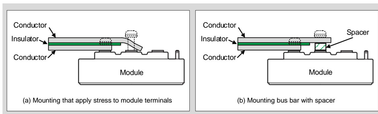
Fig. 4-6 Mounting with laminated bus bar
