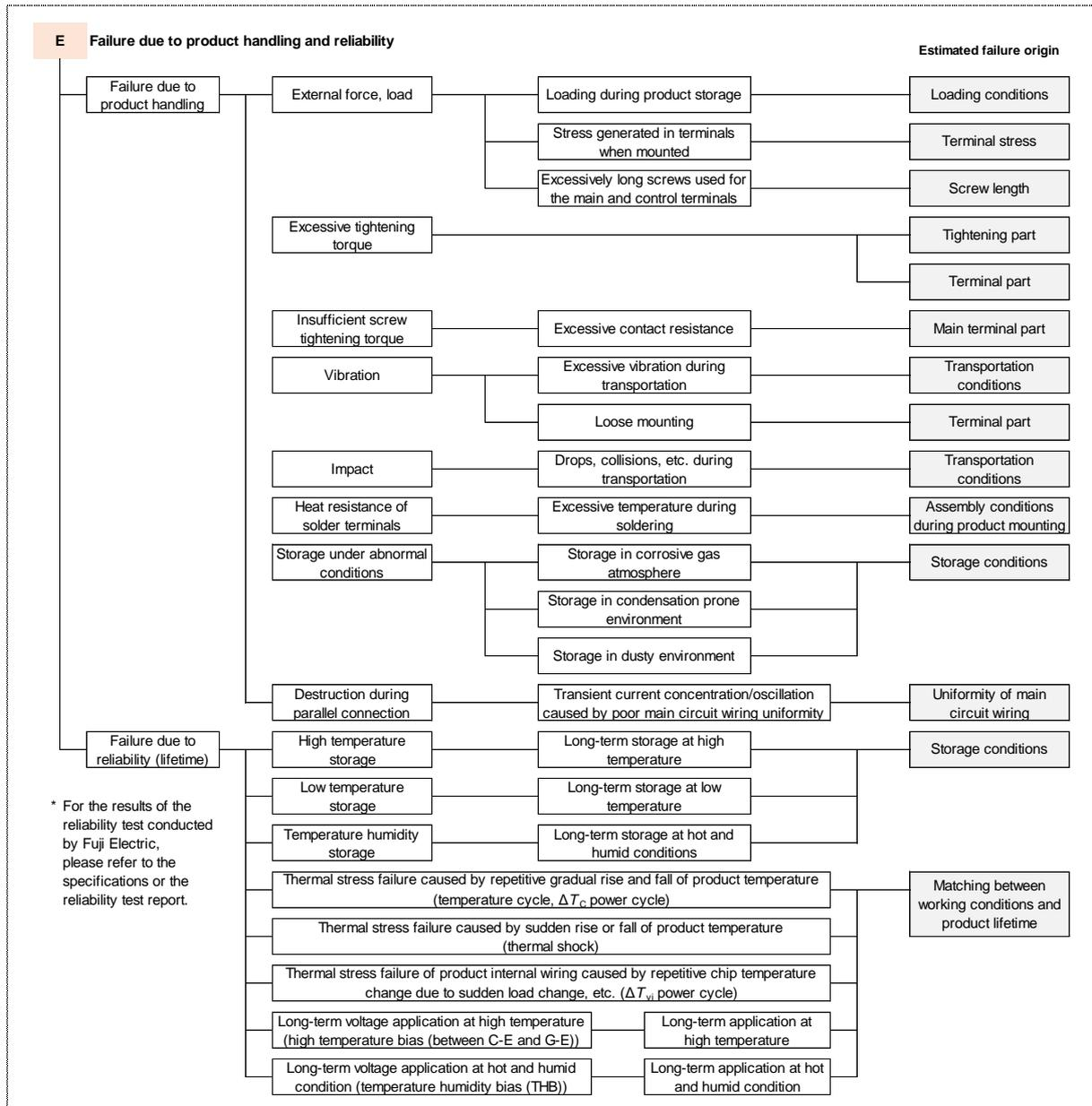
Fig. 4-1(f) Mode E: Failure due to product handling and reliability
