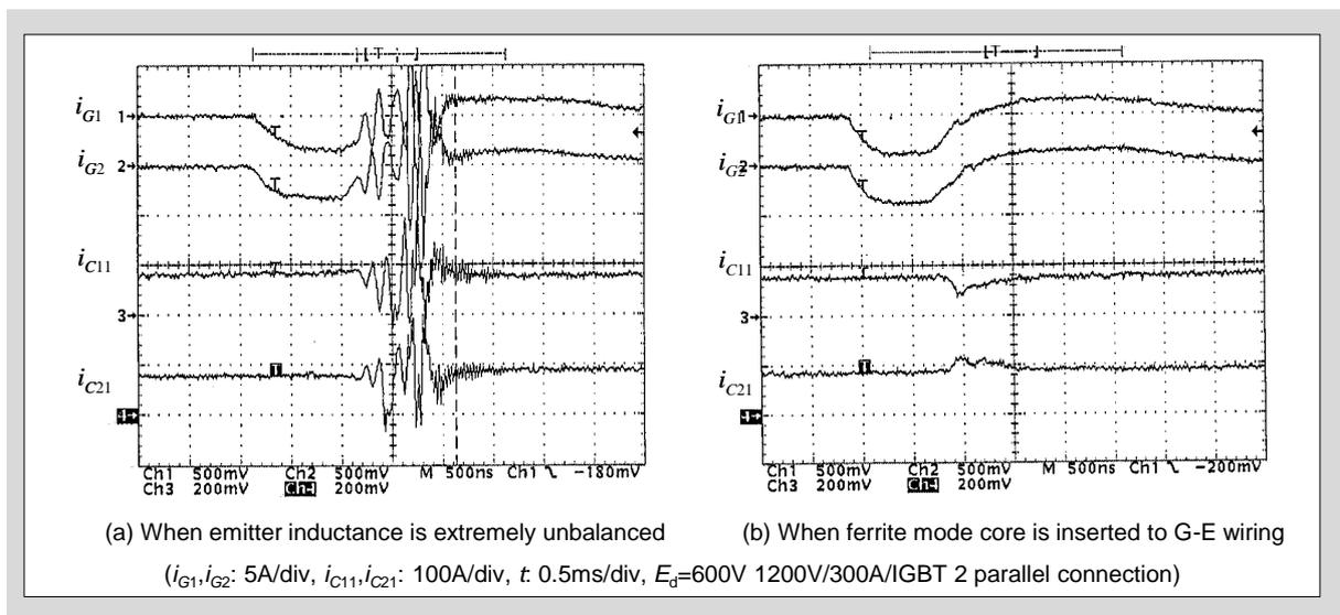
Fig. 4-10 Waveforms of 2 parallel connection
