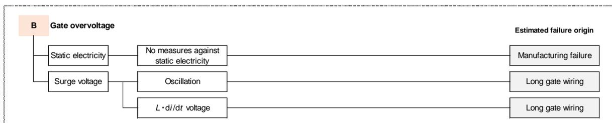
Fig. 4-1(c) Mode B: Gate overvoltage
