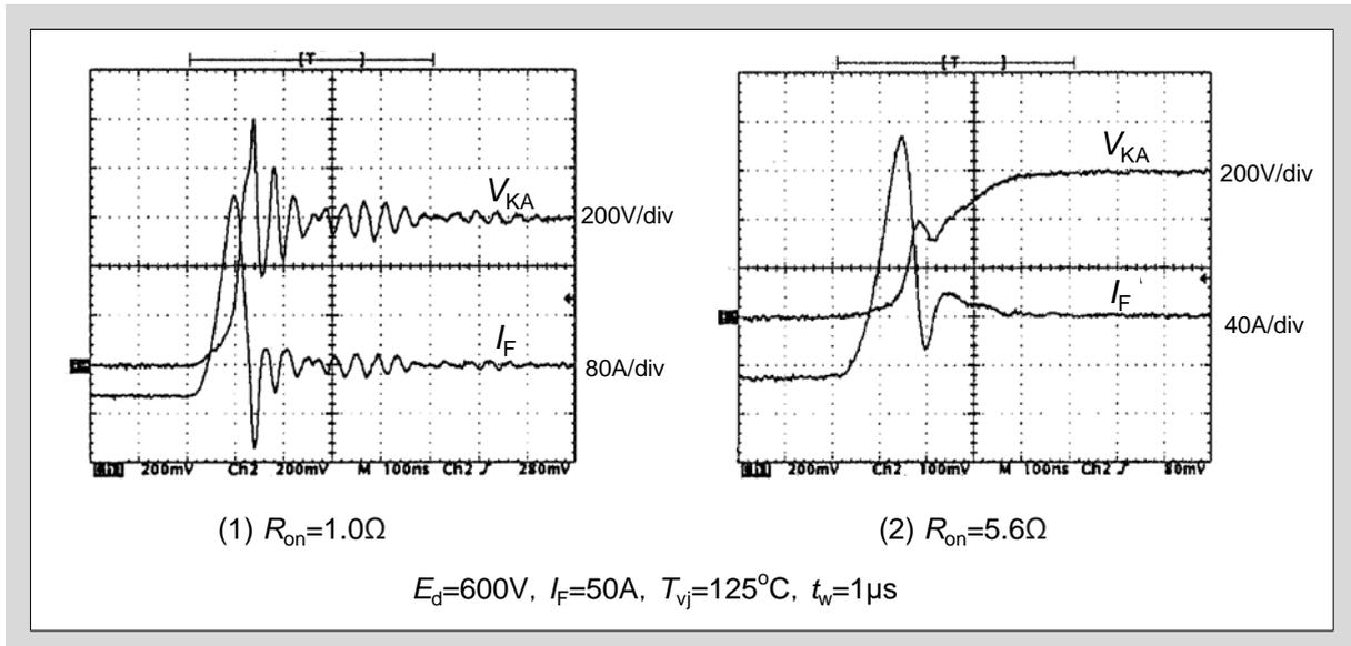
Fig. 4-9 Waveforms of short on-pulse reverse recovery
