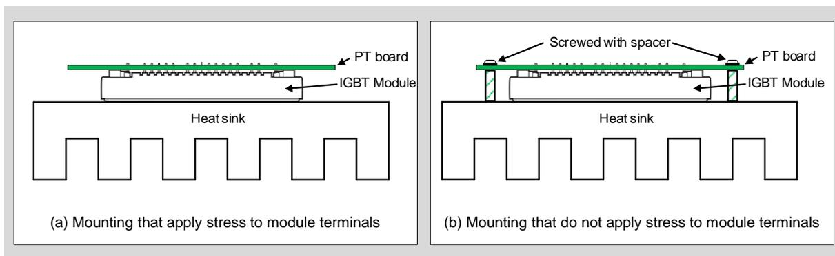
Fig. 4-5 Fixing a PCB
