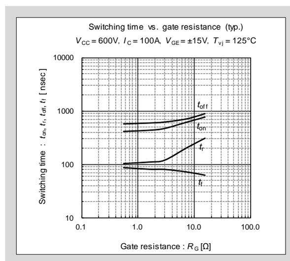
Fig. 2-8 Switching time -  $R_G$  characteristics
