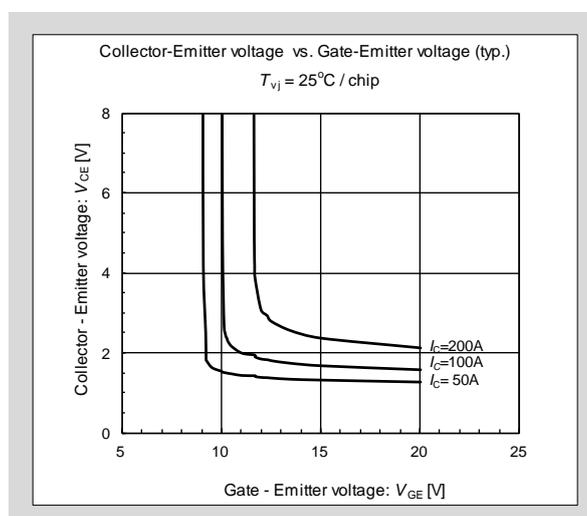
Fig. 2-3  $V_{CE} - V_{GE}$  characteristics ( $T_{vj}=25^{\circ}C$ )
