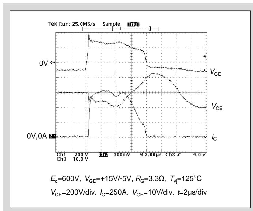
Fig. 5-5 Waveforms during short circuit protection
