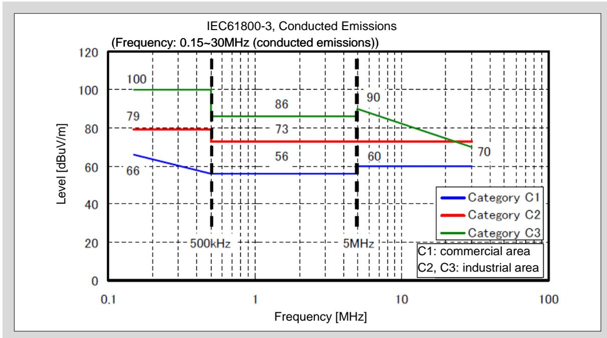
Fig. 10-2 Limits of conducted emissions in IEC61800-3
