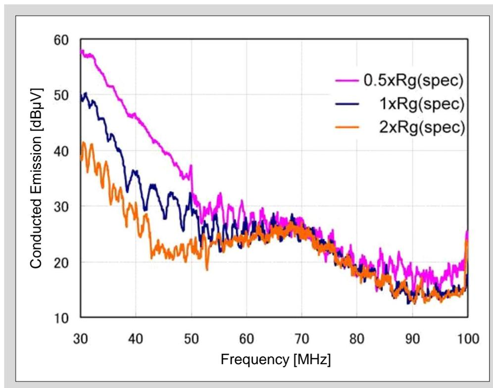
Fig. 10-28 Radiated emission dependence on gate resistance (7MBR100U4B-120)
