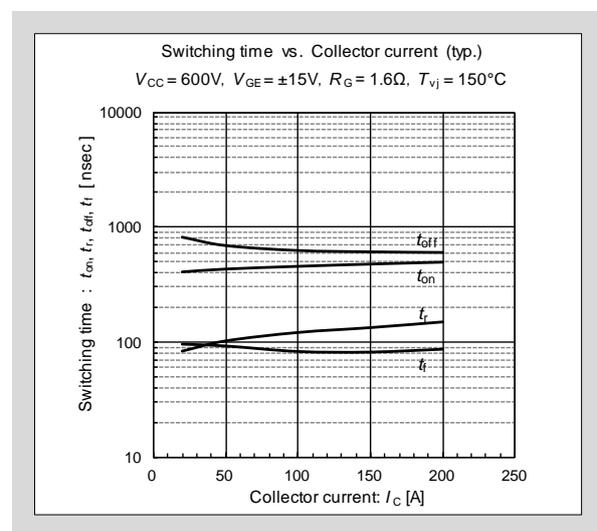
Fig. 2-7 Switching time -  $I_C$  characteristics
