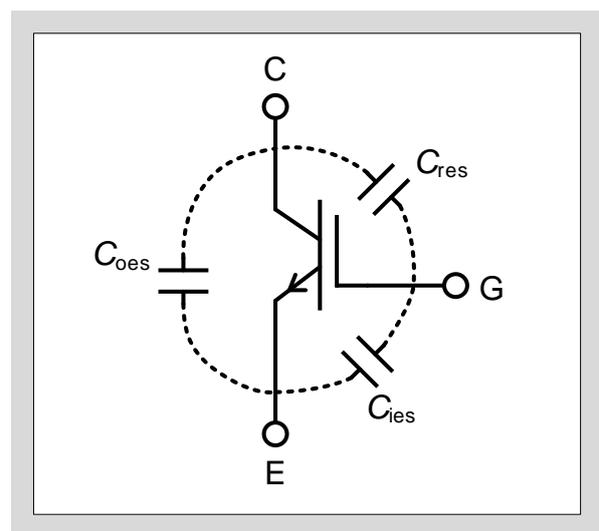
Fig. 2-13 Junction capacitance
