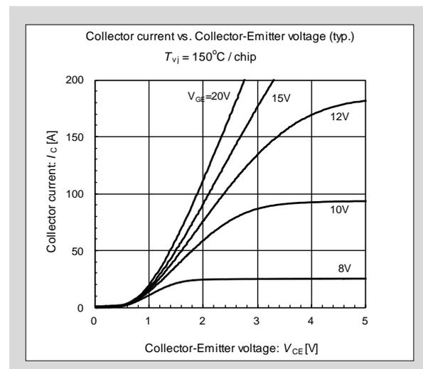
Fig. 2-2  $V_{CE(sat)} - I_C$  characteristics ( $T_{vj}=150^{\circ}C$ )
