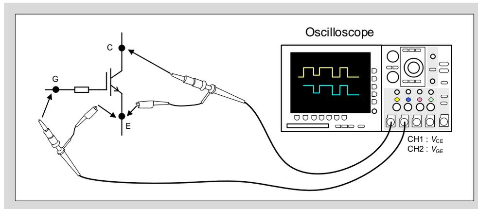
Fig. 9-10 Voltage probes connection
