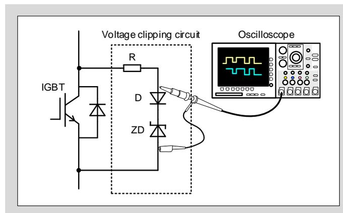
Fig. 9-1 Measurement method of saturation voltage
