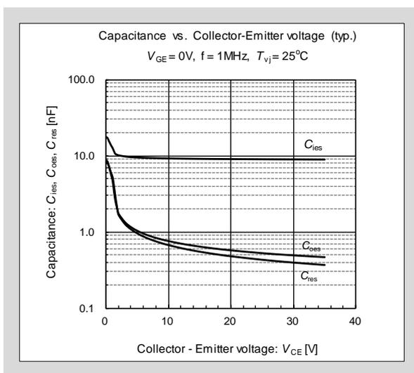
Fig. 2-12 Junction capacitance characteristic
