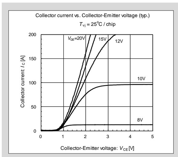
Fig. 2-1  $V_{CE(sat)} - I_C$  characteristics ( $T_{vj}=25^{\circ}C$ )
