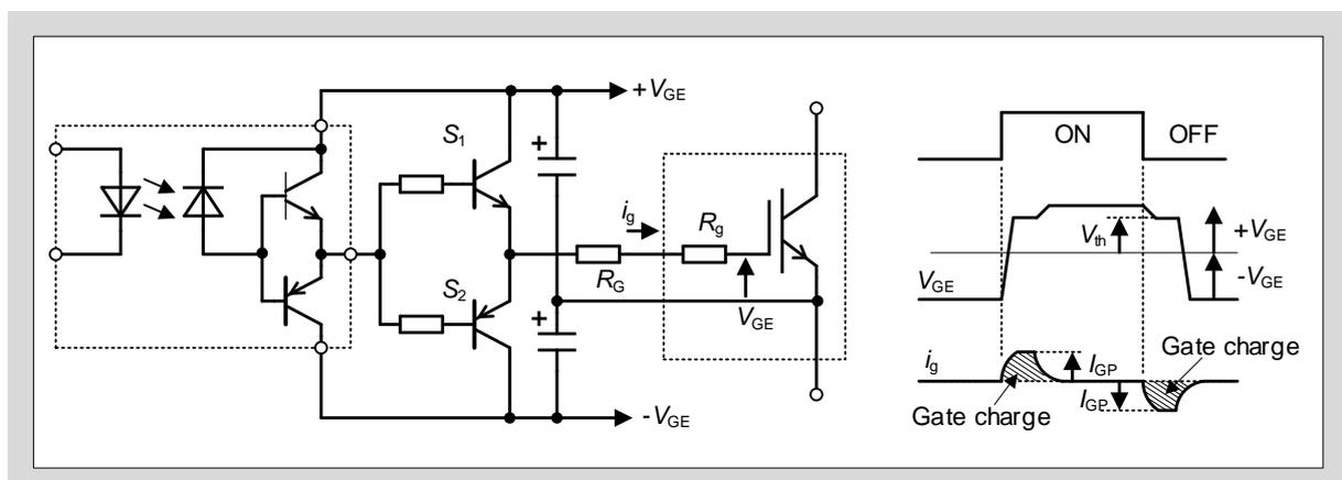
Fig. 7-4 Gate drive circuit schematic and waveforms
