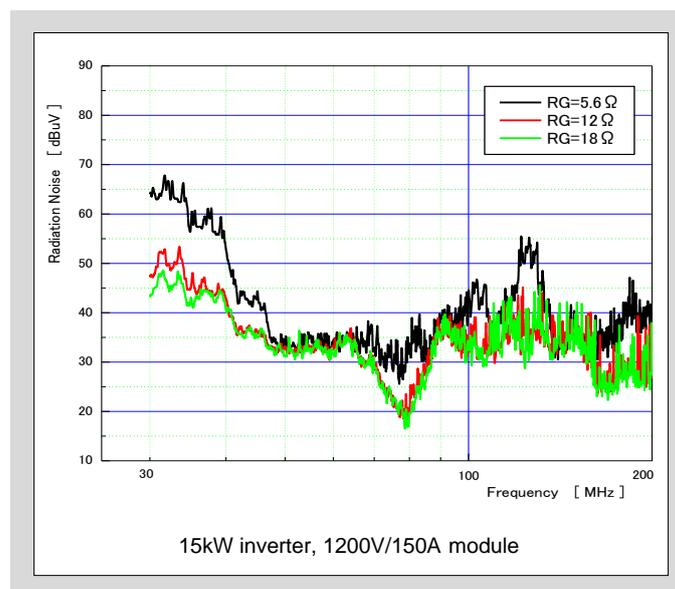
Fig. 4-11 Radiation noise ( $R_G$  dependence)
