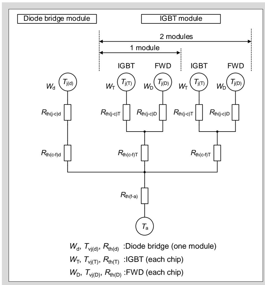
Fig. 6-10 Thermal resistance equivalent circuit
