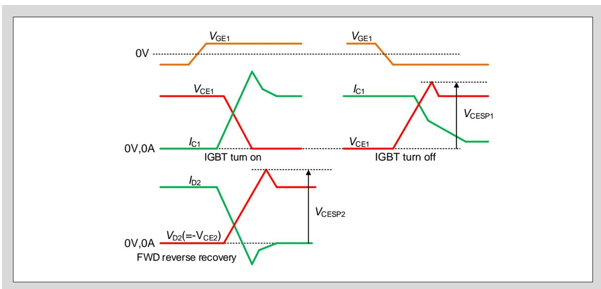
Fig. 5-7 Switching waveforms
