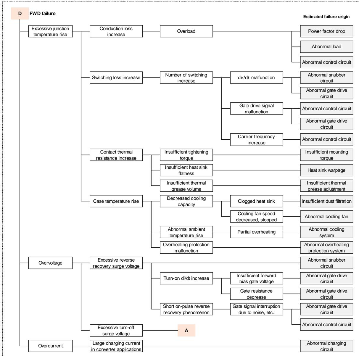
Fig. 4-1(e) Mode D: FWD failure
