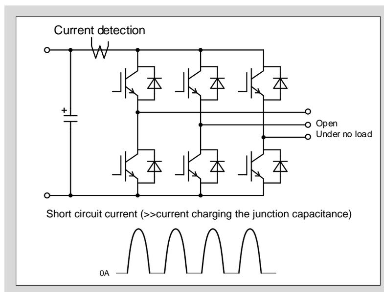
Fig. 4-7 Short circuit current measuring circuit
