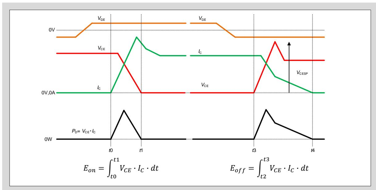
Fig. 9-5 Switching loss
