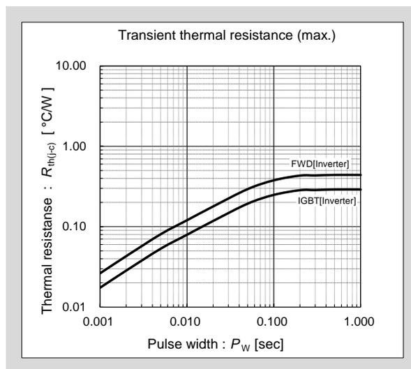
Fig. 2-17 Transient thermal resistance
