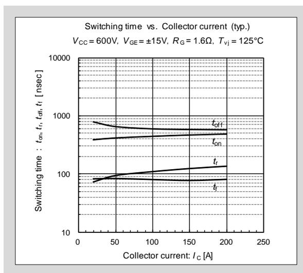
Fig. 2-6 Switching time -  $I_C$  characteristics
