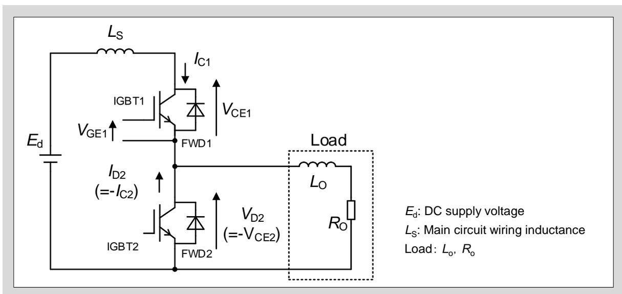
Fig. 5-6 Chopper circuit
