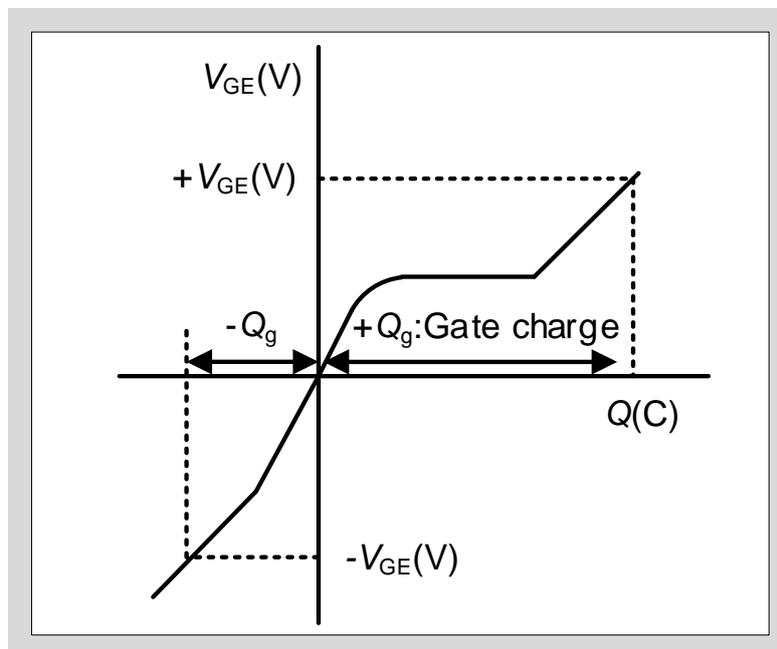
Fig. 7-3 Gate charge (Dynamic input) characteristics
