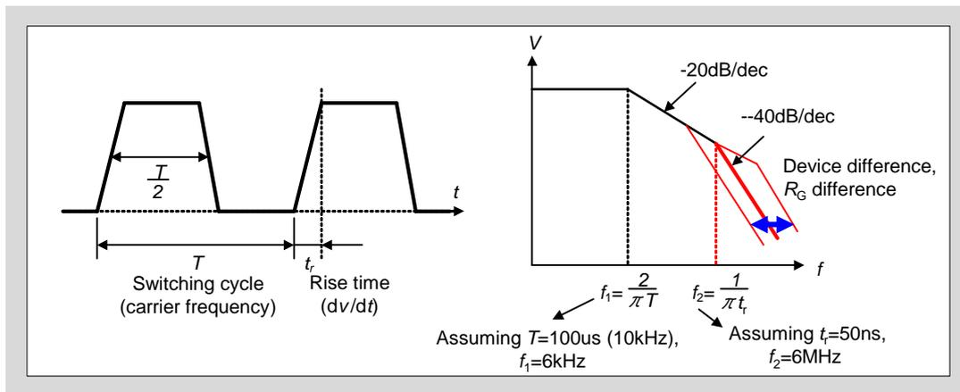
Fig. 10-14 IGBT voltage waveform and frequency spectrum
