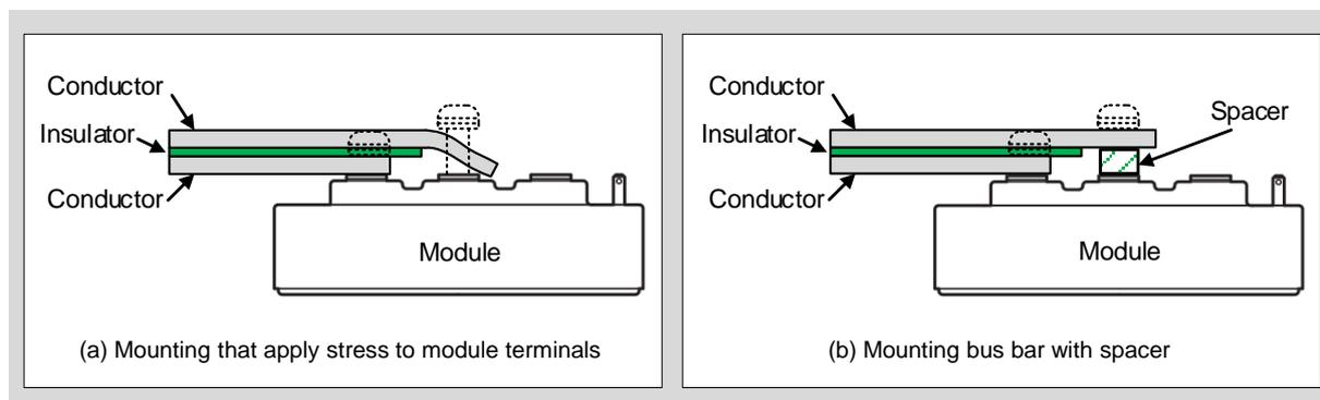
Fig. 4-6 Mounting with laminated bus bar
