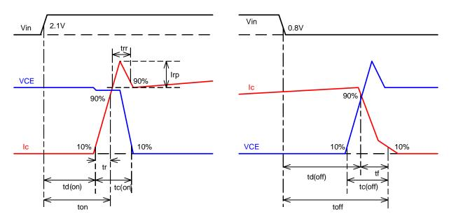
Fig.2-1 Switching waveforms
