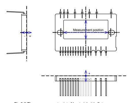
Fig.2-3 The measurement point of heat-sink side flatness.
