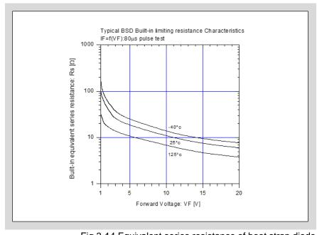
Fig.3-14 Equivalent series resistance of boot strap diode
