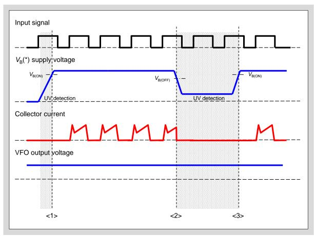
Fig.3-5 Operation sequence of  $V_{\rm B}(^*)$  Under voltage protection (high side)
