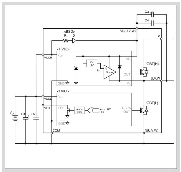
Fig.3-4 UV protection circuit of  $V_B(U, V, W)$
