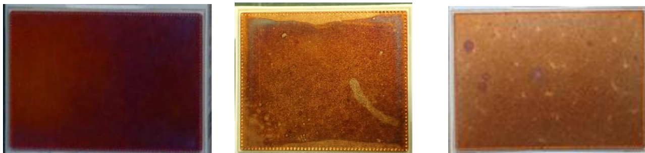
Figure 15 examples of discoloration on mounting surfaces which do not affect the thermal behavior
