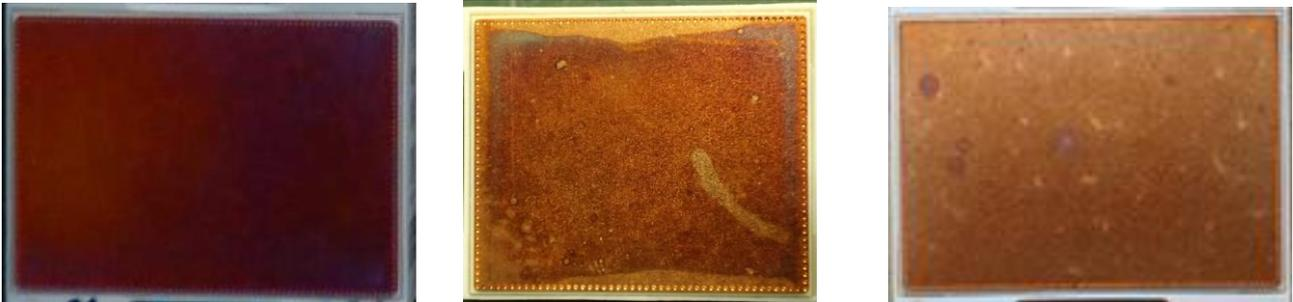
Figure 8 examples of discoloration on mounting surfaces which do not affect the thermal behavior
