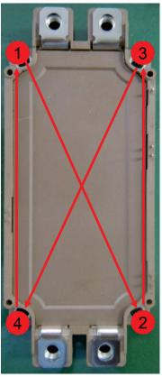
Fig.12 Mounting holes (1) ~ (4) in Press Fit module
