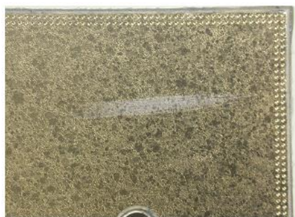
Fig.4 Bottom Surface NiAu DCB after rework
