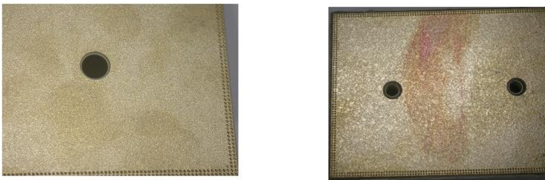
Fig.3 NiAu DCB with fingerprints or discoloration
