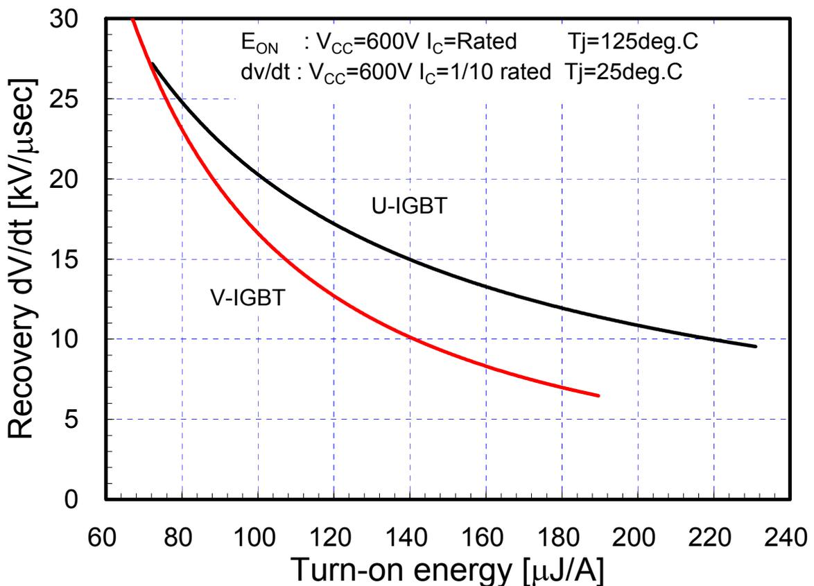
Fig. 3-5 Relation between Reverse Recovery dV/dt and Turn-on Loss (1200V series)
