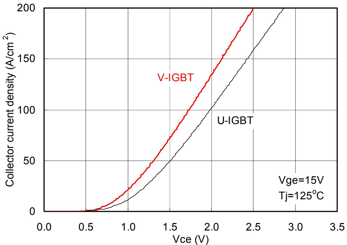
Fig. 3-1 Comparison of Output Characteristics (1200V series)
