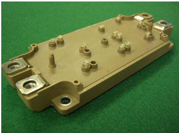
Fig. 6-1 Spring contact module
