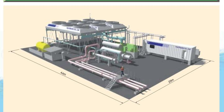
Equipment, piping and cables are functionally arranged in consideration with sufficient operation and maintenance spaces.
