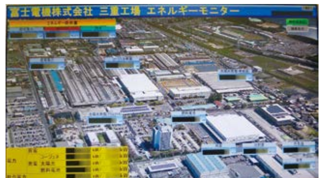
Energy data tracking monitor (total electricity consumption)
