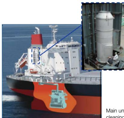
Main unit of ship exhaust gas cleaning system (upper right)
