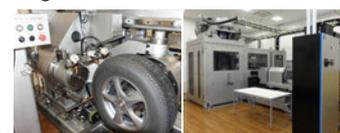
Tire testing machine compatible with WLTP
