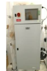
Water quality meter (pH, PAH, turbidity)
