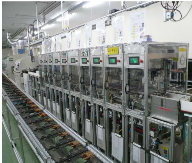
Automated smart meter assembly line
