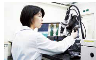
Sample observation using digital microscope with up to 5,000x magnification
