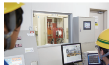
Breaking test to verify safety during large current flow accidents
